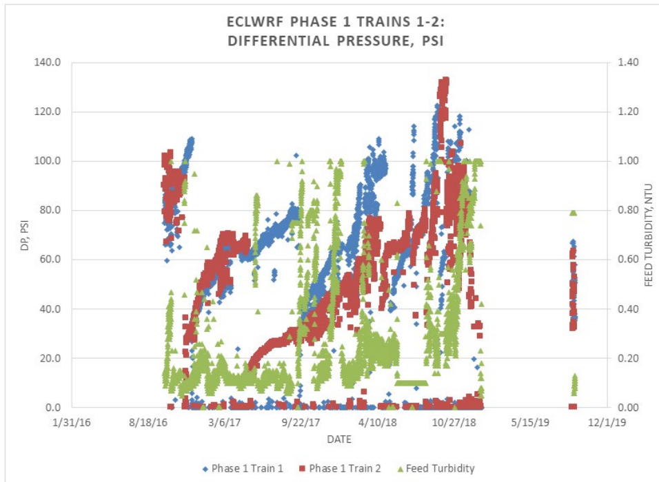
Figure 4-41. ECLWRF Barrier RO Trains 1 and 2 Differential Pressure and Feed Turbidity
