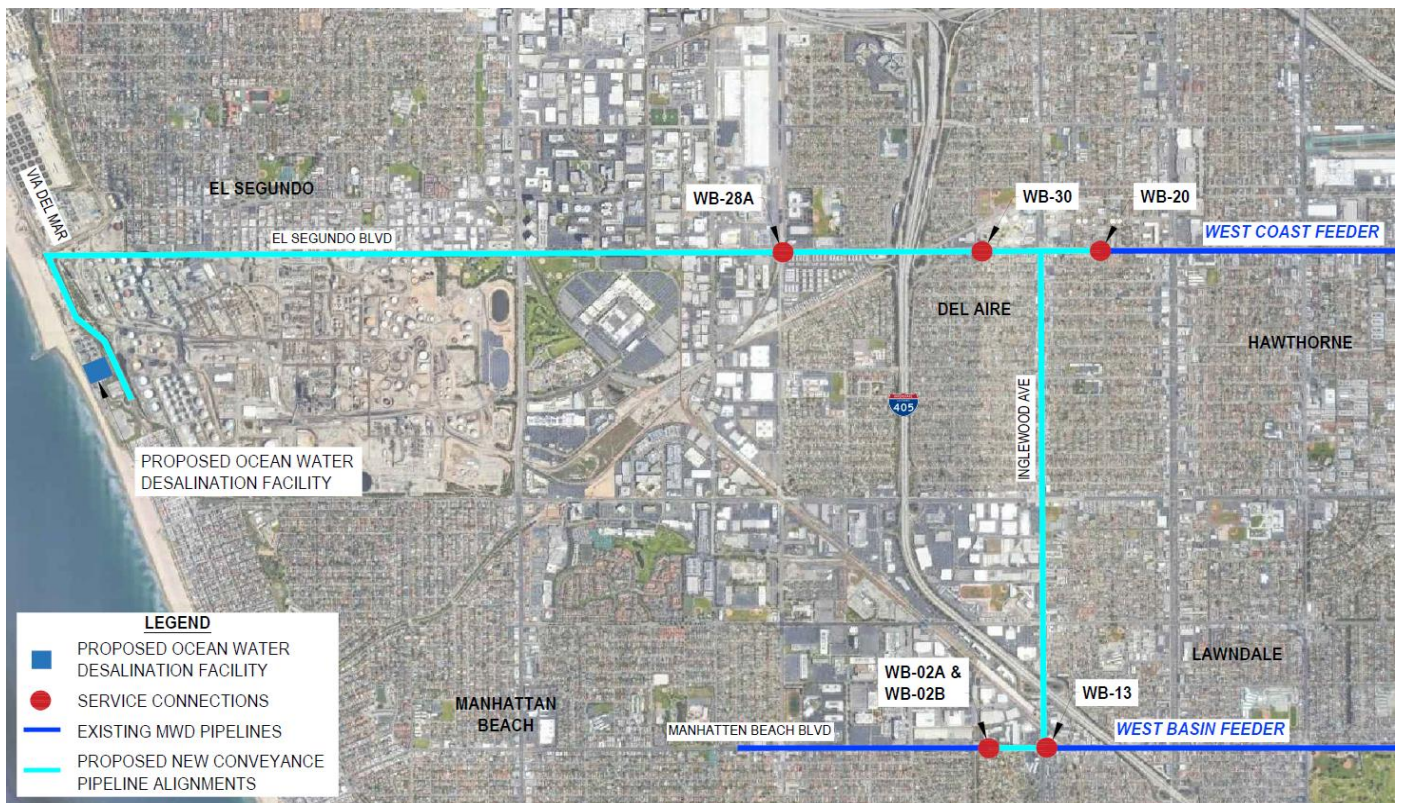
Figure II-3 Desalinated Water Conveyance Recommended Alignment
