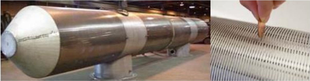
Figure II-7 Typical (Cylindrical) Wedge Wire Screen Design
