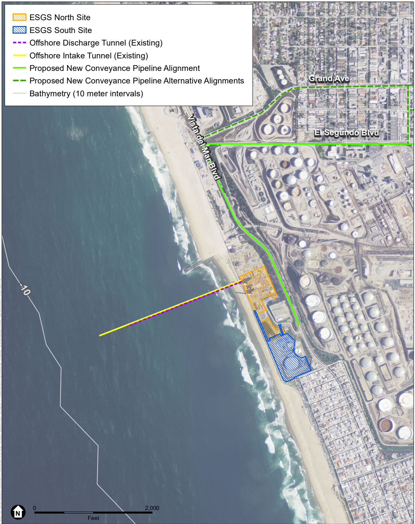
Figure 3-4 Existing 12-foot Diameter Intake and Discharge Tunnels
