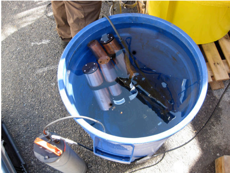
Figure D3. WQM submerged in water for testing
