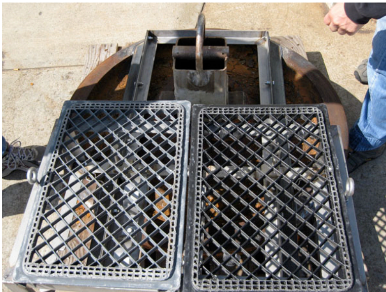
Figure D10. RR Wheel Anchor with plastic cover for WQM cage and ring for chain mooring
