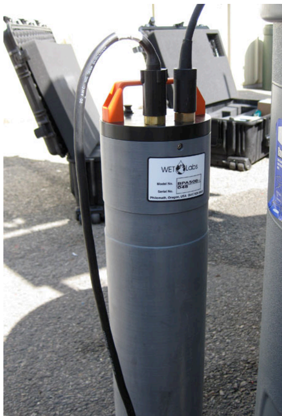
Figure D4. Battery for WQM located at ocean bottom (15 m depth)
