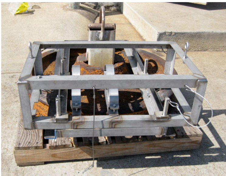
Figure D9. RR Wheel Anchor and mounting for WQM at depth (15 m)
