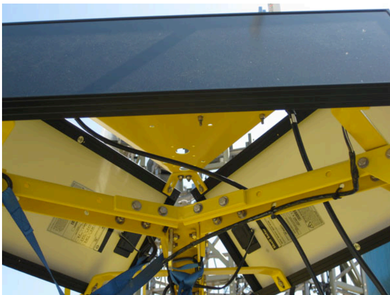
Figure D8. Solar panels on top of buoy
