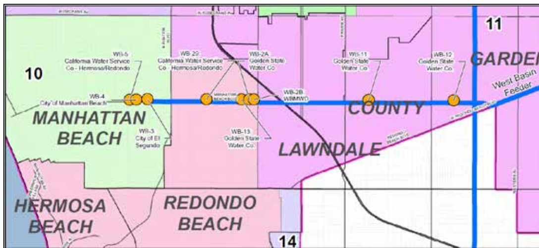
Figure 2-5: MWD Service Connections along West Basin Feeder
