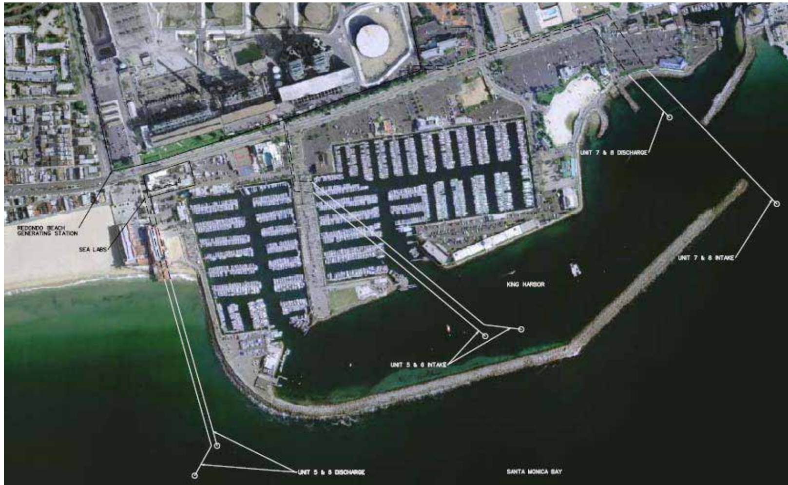
Figure 4-3: Redondo Beach, Existing Intake and Discharge Layout Source: MWH "Redondo Beach Generating Station Overview", 2006.
