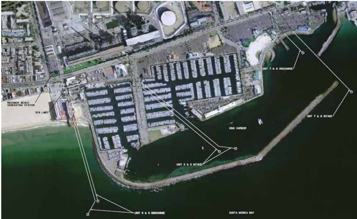
Figure 4. AES Redondo Beach tunnels layout.
