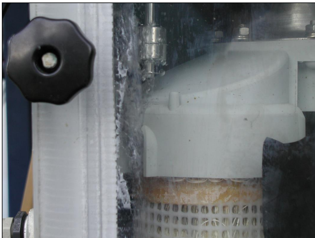
Figure 6-7 Air Bubbles Emitted from the Cracked Epoxy During the Pressure Decay Test
