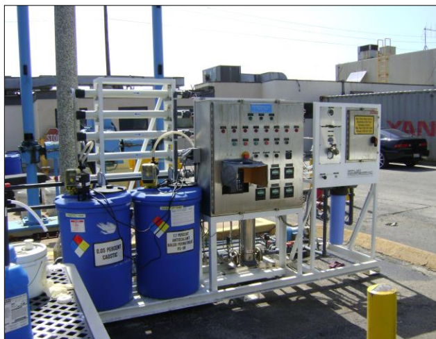
Figure 1-4 Second Pass RO System
