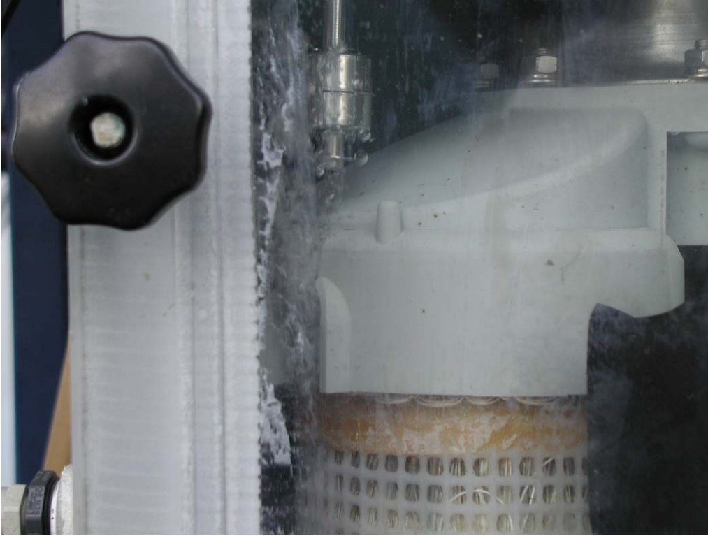
Figure 11 - Air Bubbles Emitted from the Cracked Epoxy During the Pressure Decay Test
