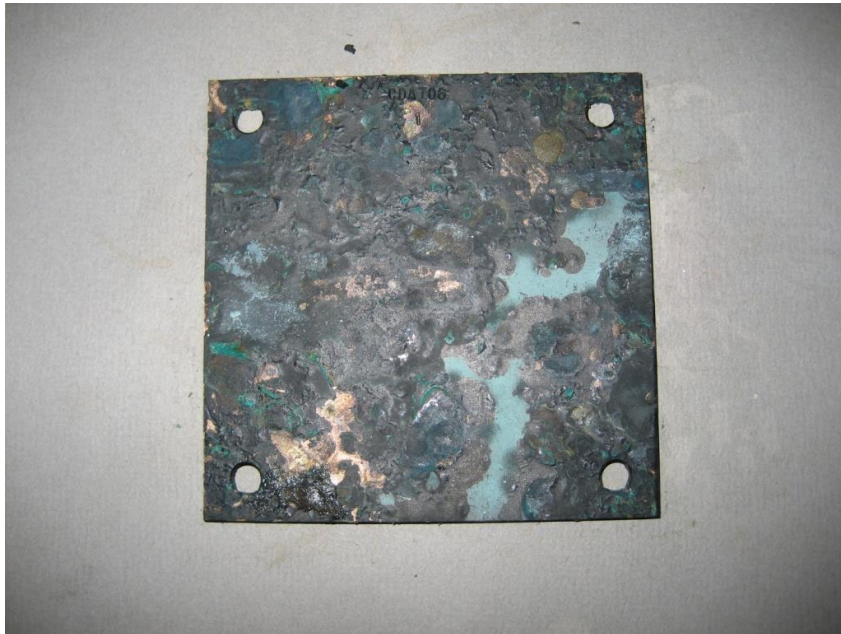
Figure 4-16: 90/10 Cu-Ni (CDA706) test plate (Test Plate 1), photographed 06/18/15 prior to biofouling inspection.
