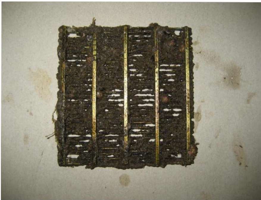
Figure 4-14: 70-30 Cu-Ni (CDA715) wedgewire sample, photographed 05/24/17.
