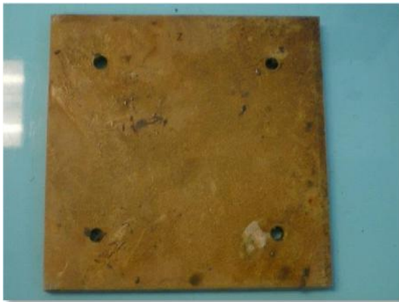
Figure 4-42: Minimal corrosion was observed on the Z alloy flat plate.
