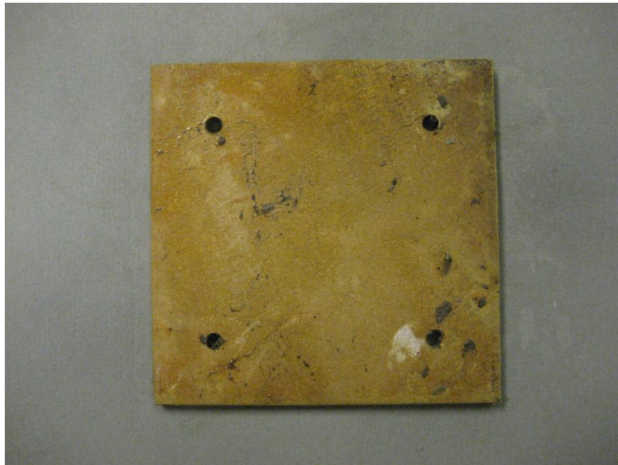
Figure 4-18: Z-alloy test plate (Test Plate 3), photographed 06/18/15 prior to biofouling inspection.
