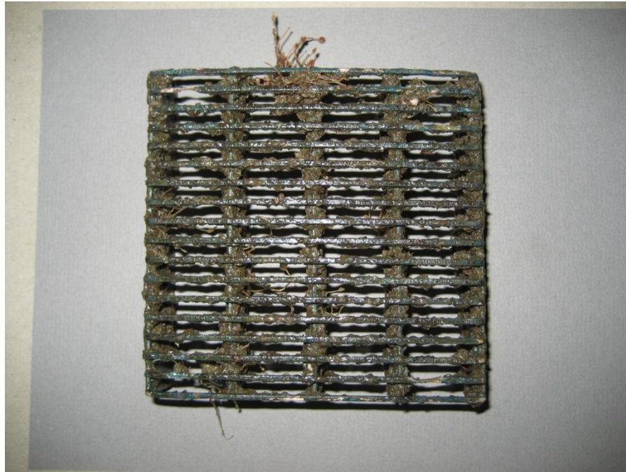
Figure 4-1: 90/10 Cu-Ni (CDA706) Wedgewire sample, photographed 06/17/15.
