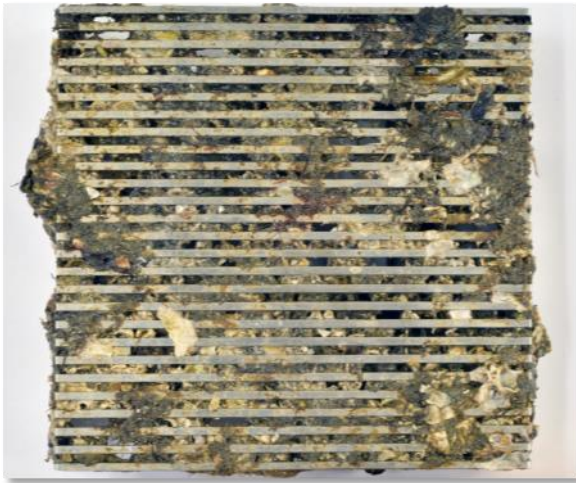
Photo 4-1: Uncoated 2205 Duplex SS wedgewire screen, before cleaning.
