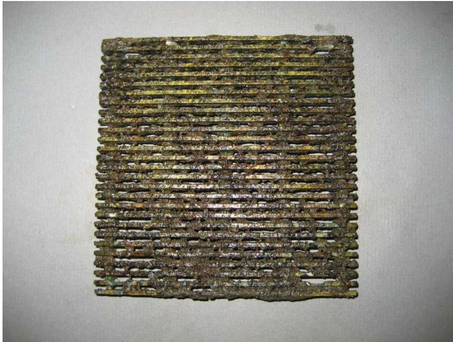
Figure 4-9: 70/30 Cu-Ni (CDA715) Wedgewire sample, photographed 06/17/15.
