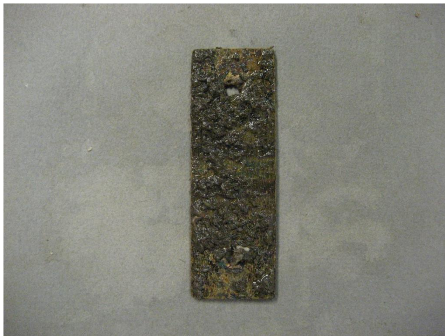
Figure 4-2: 90/10 Cu-Ni (CDA706) coupon, photographed 06/17/15.
