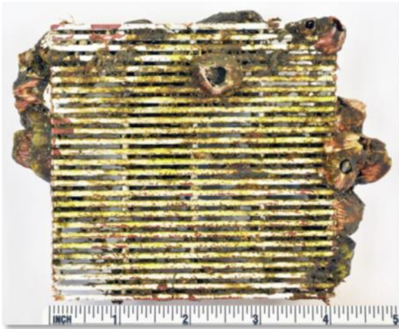
Photo 4-5: Coated 2205 Duplex SS wire screen, before cleaning.
