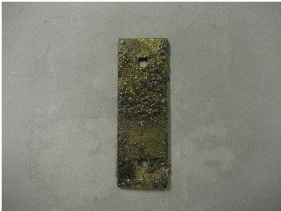
Figure 4-10: 70/30 Cu-Ni (CDA715) coupon, photographed 06/17/15.
