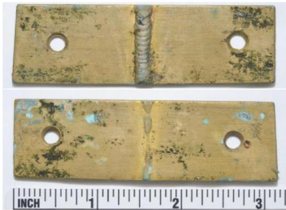
Figure 4-40: Surface discoloration of Z alloy coupon, front (top), back (bottom).
