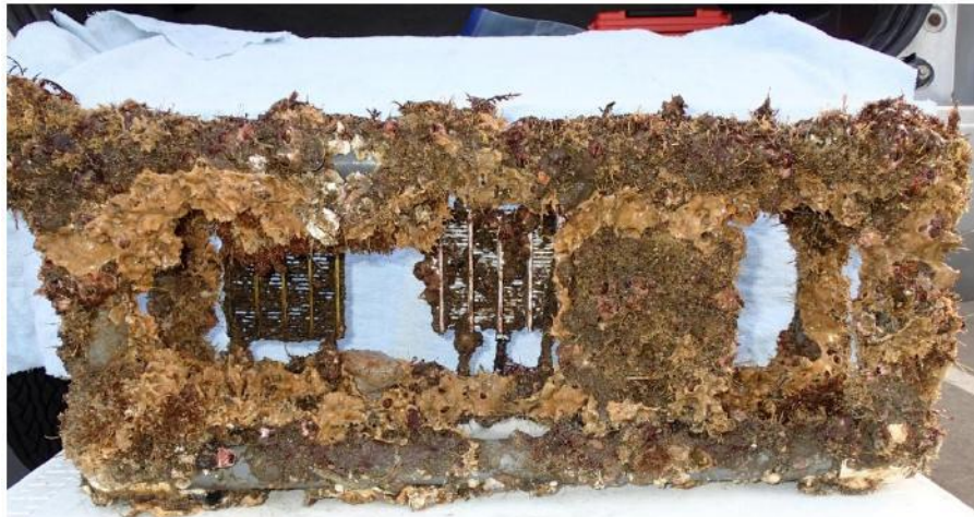
Figure 4-11: Rack V with three remaining wedgewire samples still attached, photographed 05/23/17.
