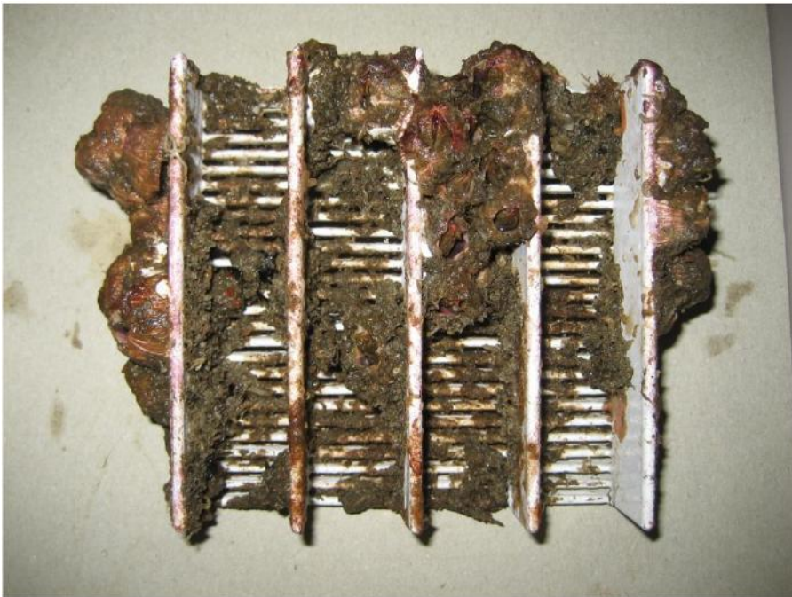
Figure 4-12: 2205 stainless steel wedgewire sample with foul release coating, photographed 05/24/17.
