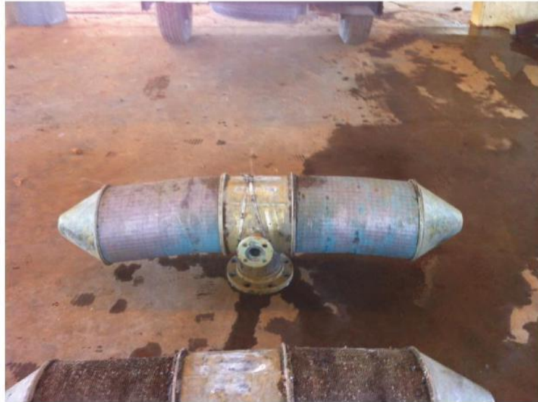
Cook Legacy Screen after Structural Failure
