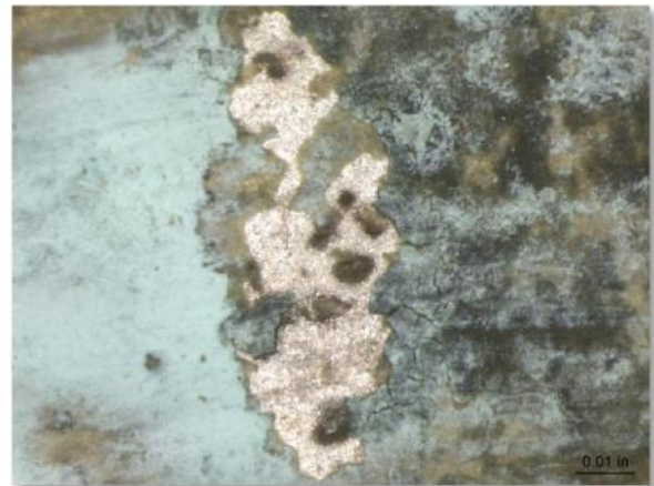
Figure 4-41: Surface discoloration of Z alloy coupon, shown at 50X magnification.
