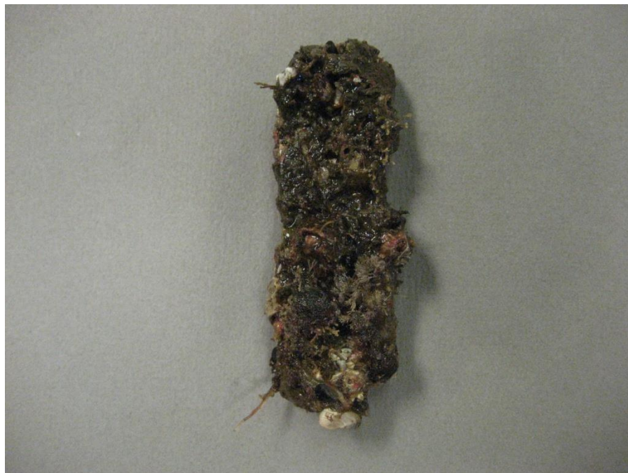
Figure 4-8: 2205 stainless steel coupon, photographed 06/17/15.
