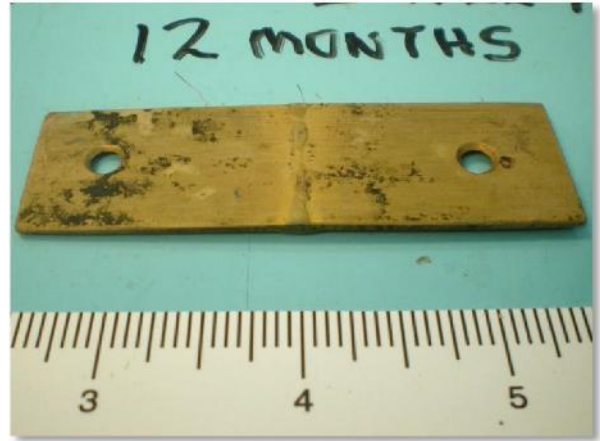
Figure 4-39: Z alloy 1-inch by 3-inch coupon with weld front.
