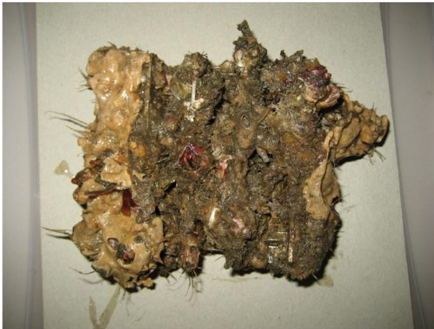
Figure 4-13: 2205 stainless steel wedgewire sample, photographed 05/24/17.
