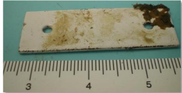
Figure 4-27: Slight damage to coating on edge and initiation of biofouling on corner of coated 2205 Duplex stainless steel coupon.
