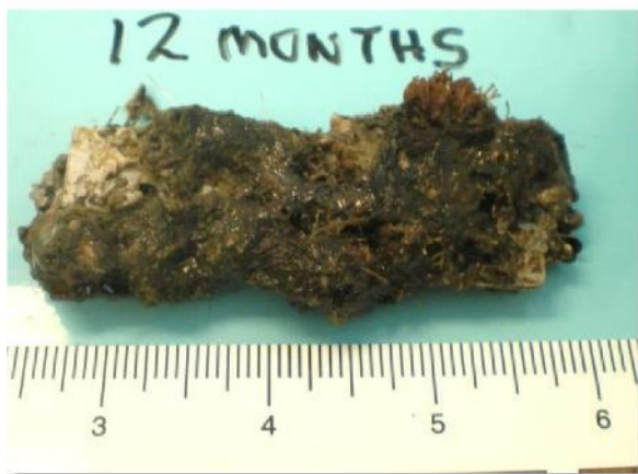
Figure 4-24: Marine life attached to uncoated 2205 Duplex stainless steel coupon with a weld.
