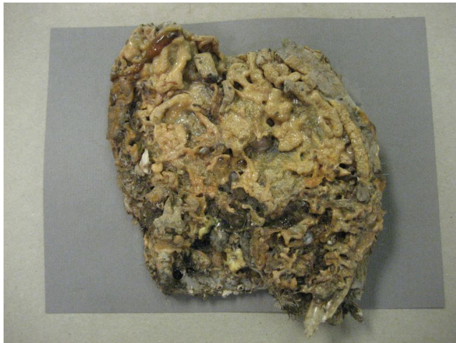
Figure 4-19: 2205 stainless steel test plate (Test Plate 4), photographed 06/18/15 prior to biofouling inspection.
