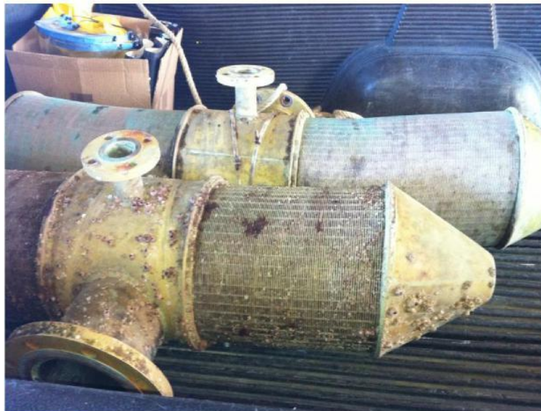
Cook Legacy Screens Removed after Failure
