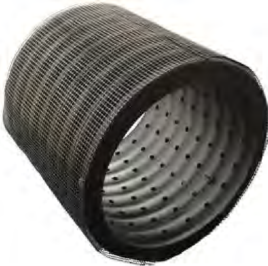
Figure 2.2: Section of 0.6 m diameter perforated lateral branch pipe used in the Fukuoka Seabed Infiltration Gallery Intake, referred to as “ Toyo Drains ”. The infiltration holes are large in comparison to the micron-scale infiltration holes of the Neodren horizontal well technology.
