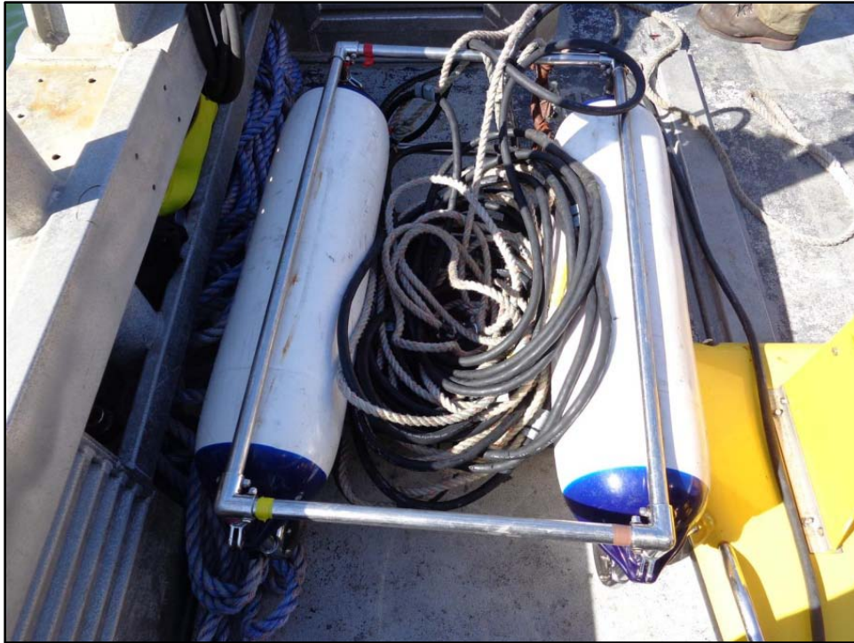
Figure 6. Boomer system (boomer plate is underneath coil of line and cable)
