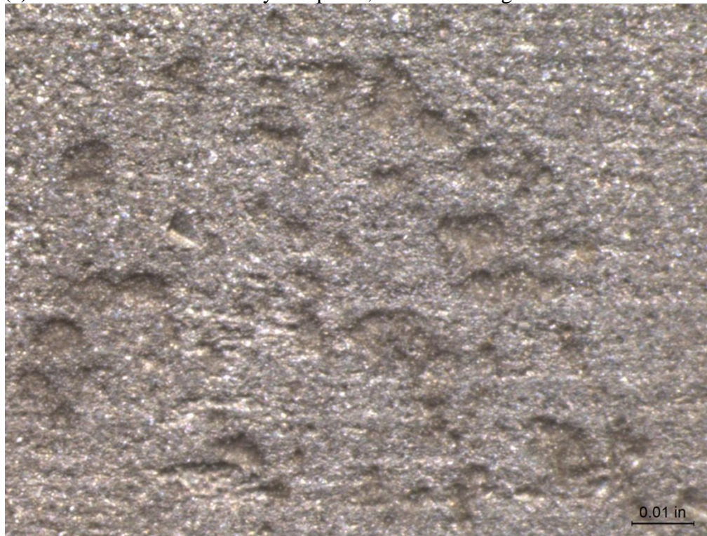
(b) Z-Alloy Coupon 4, After Cleaning 50X
