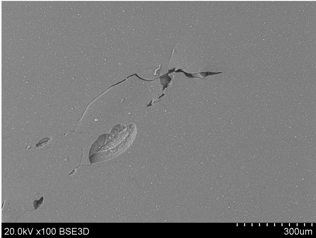
(a) Coated Duplex 2205 Stainless Steel Coupon 4, Before Cleaning 100X
