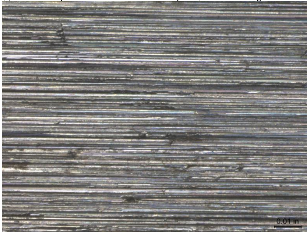
(b) Duplex 2205 Stainless Steel Coupon 6, After Cleaning 50X
