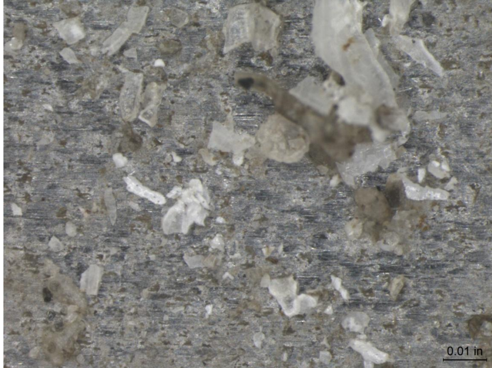
(b) Duplex 2205 Stainless Steel Plate, Before Cleaning 50X
