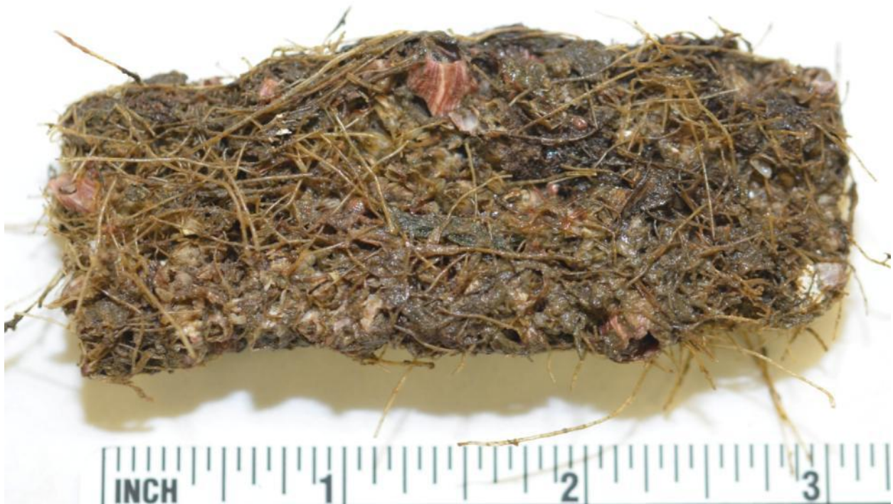
(a) Duplex 2205 Stainless Steel Coupon 6, Front Side
