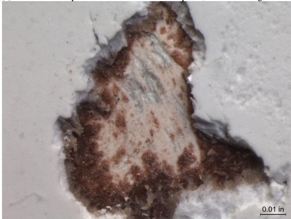
(b) Coated Duplex 2205 Stainless Steel Coupon 2, After Cleaning 50X
