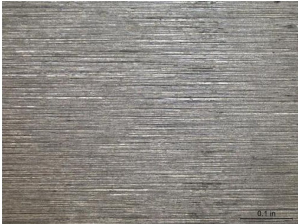
(a) CDA 715 Coupon 2, After Cleaning 10X
