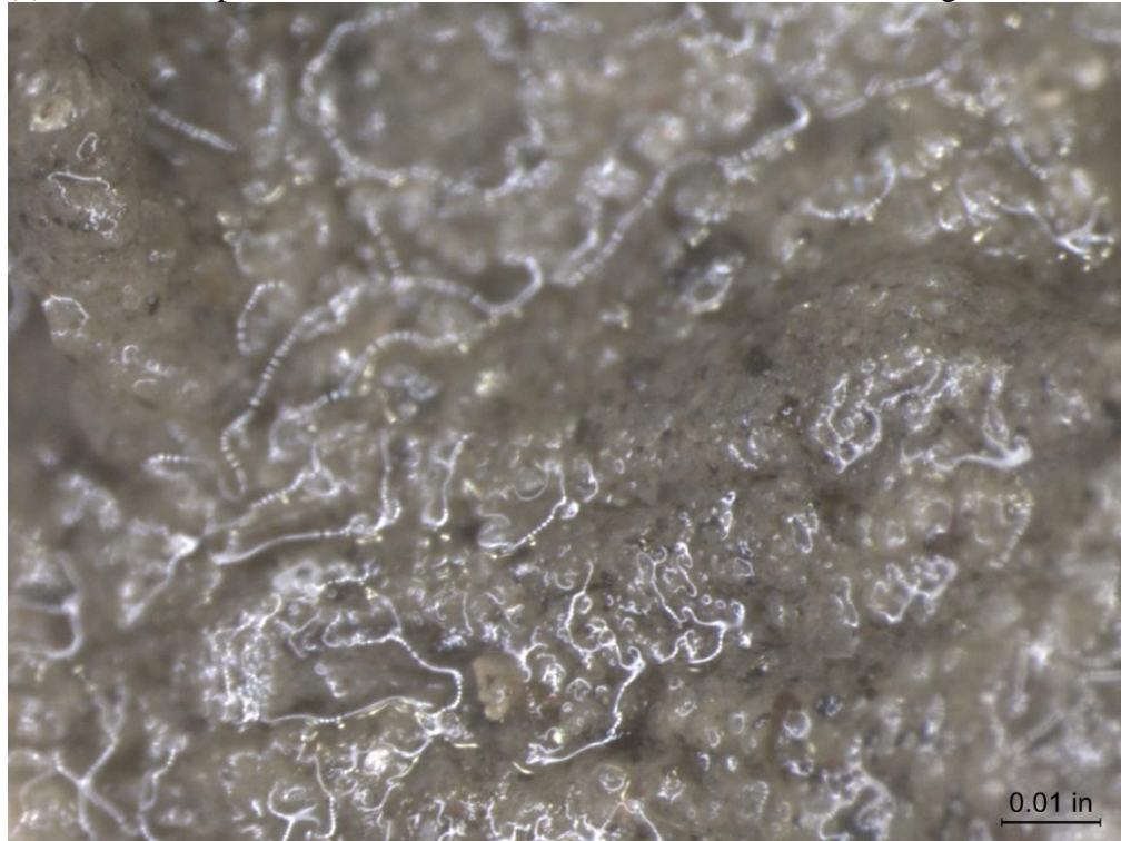
(b) Duplex 2205 Stainless Steel Screen 2, Before Cleaning 50X
