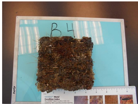
Photo 3-2. Marine life attached to uncoated 2205 Duplex stainless steel wedge wire screen.
