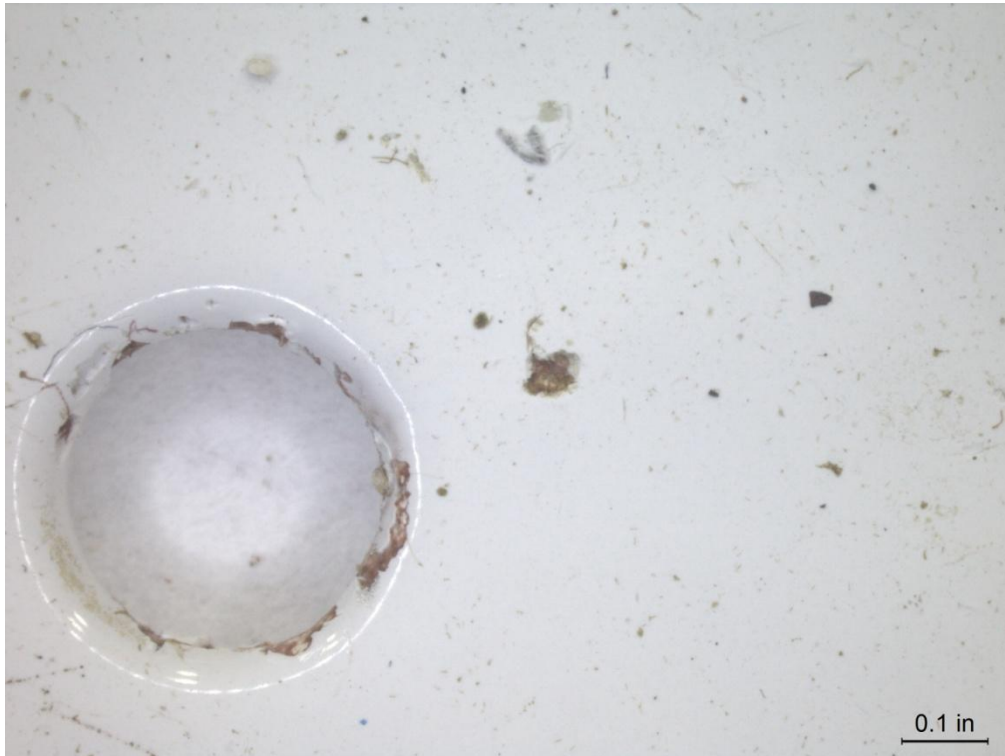
(a) Coated Duplex 2205 Stainless Steel Coupon 3, Before Cleaning 10X
