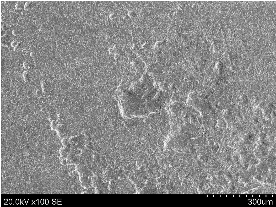
(a) Z-Alloy Coupon 1, After Cleaning 100X
