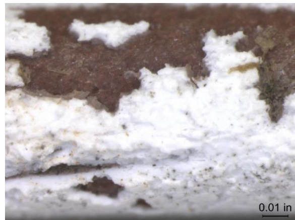
Photo 3-6. Detail view (10x) of coating damage on 2205 Duplex SS, before cleaning.
