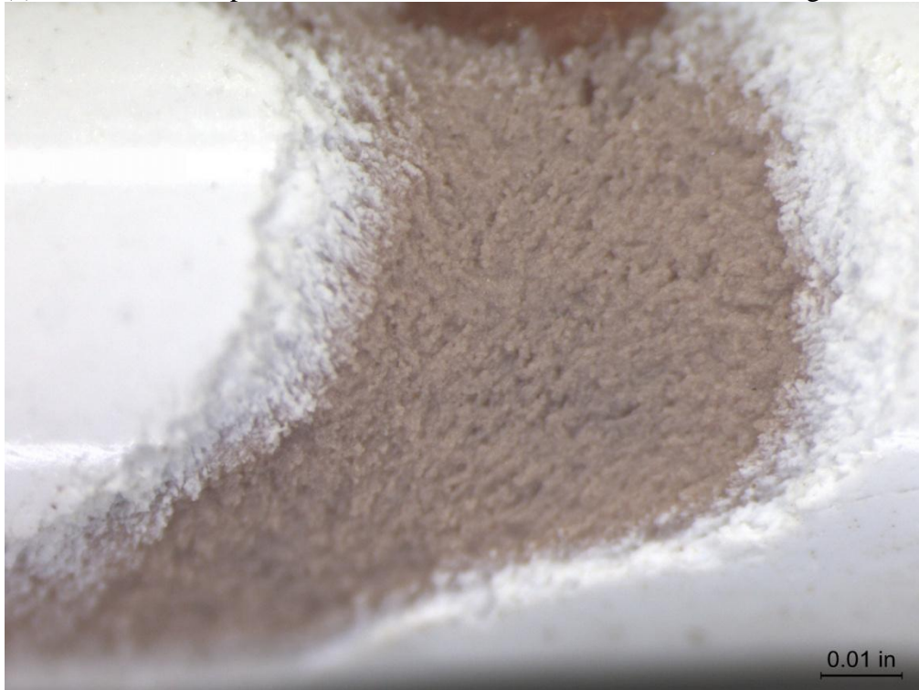
(b) Coated Duplex 2205 Stainless Steel Screen 2, After Cleaning 50X
