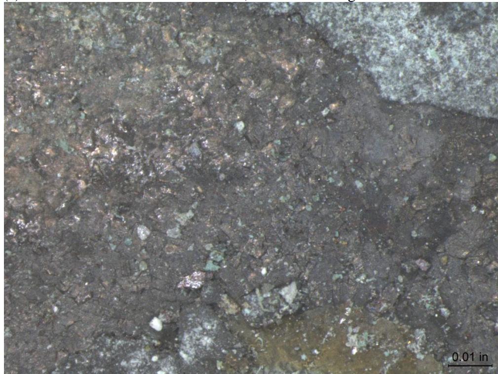
(b) CDA 706 Plate, Before Cleaning 50X
