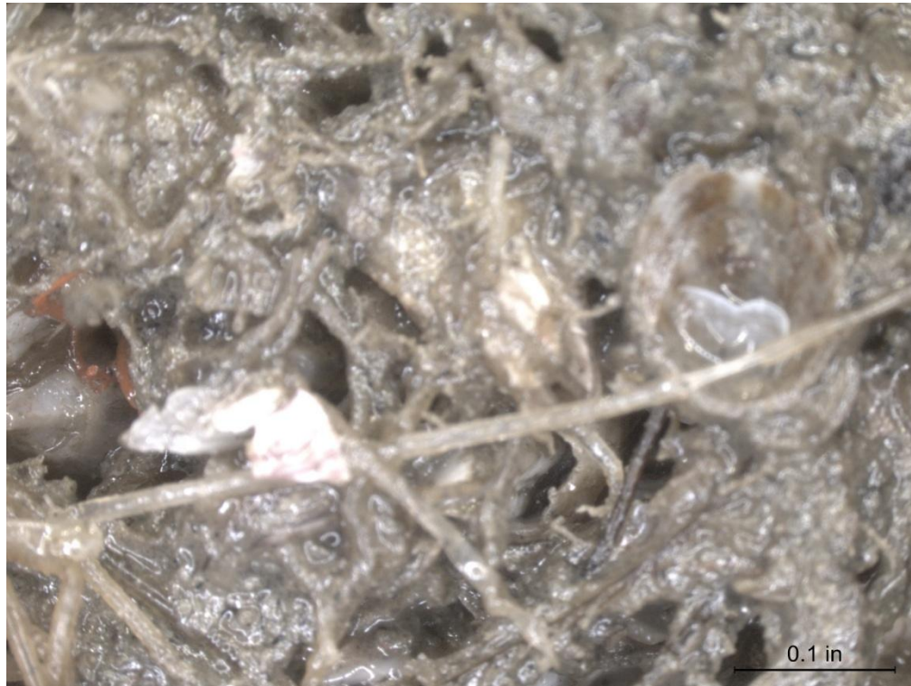
(a) Duplex 2205 Stainless Steel Coupon 7, Before Cleaning 10X
