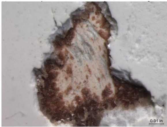
Photo 3-11. 2205 Duplex SS coupon surface exposed at an area of coating damage.
