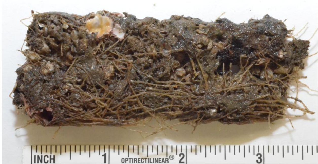
(a) Duplex 2205 Stainless Steel Coupon 7, Front Side
