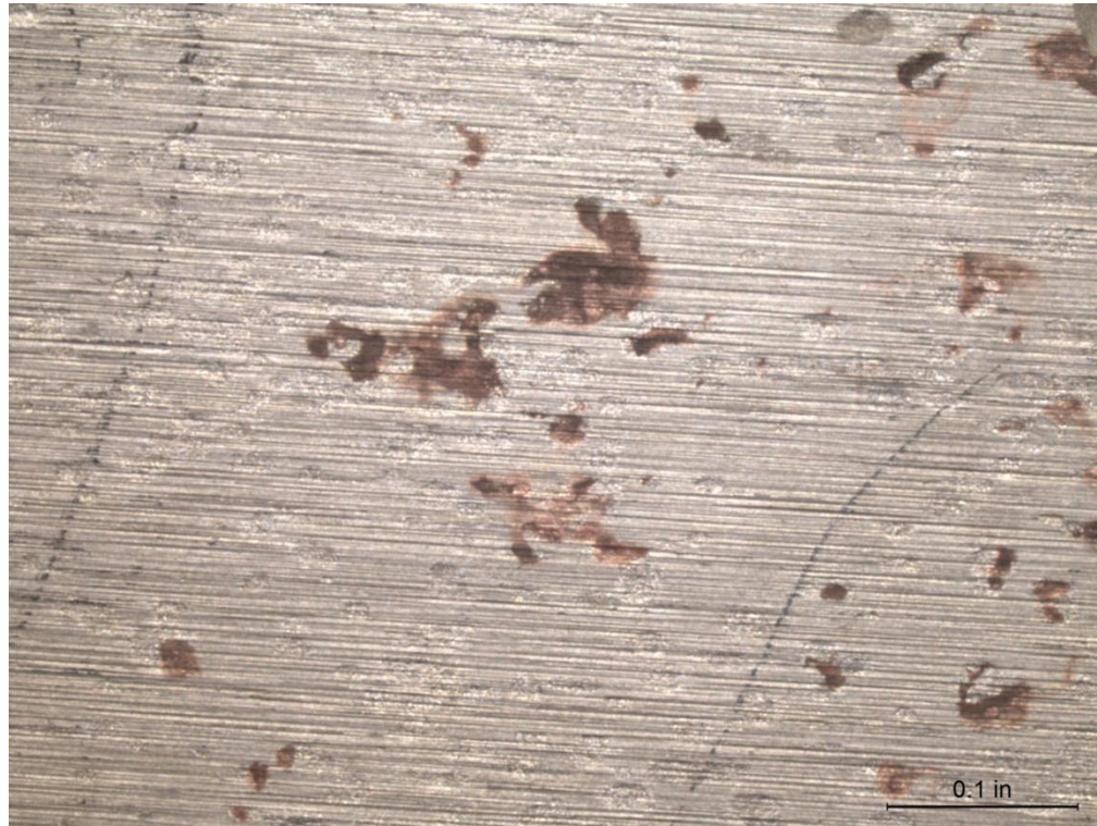
(a) CDA 706 Coupon 4, After Cleaning 10X
