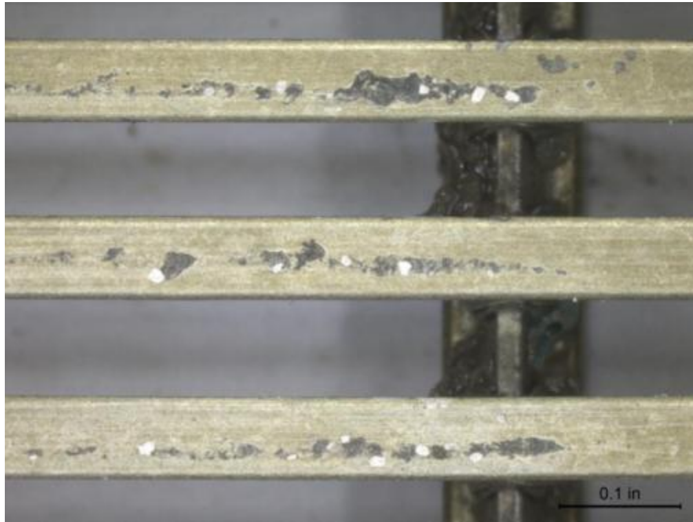
(a) CDA 715 Screen 1, Before Cleaning 10X
