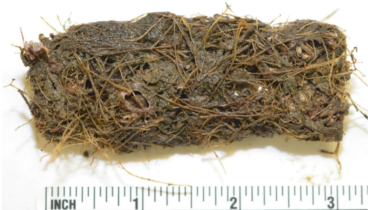
(b) Duplex 2205 Stainless Steel Coupon 6, Back Side
