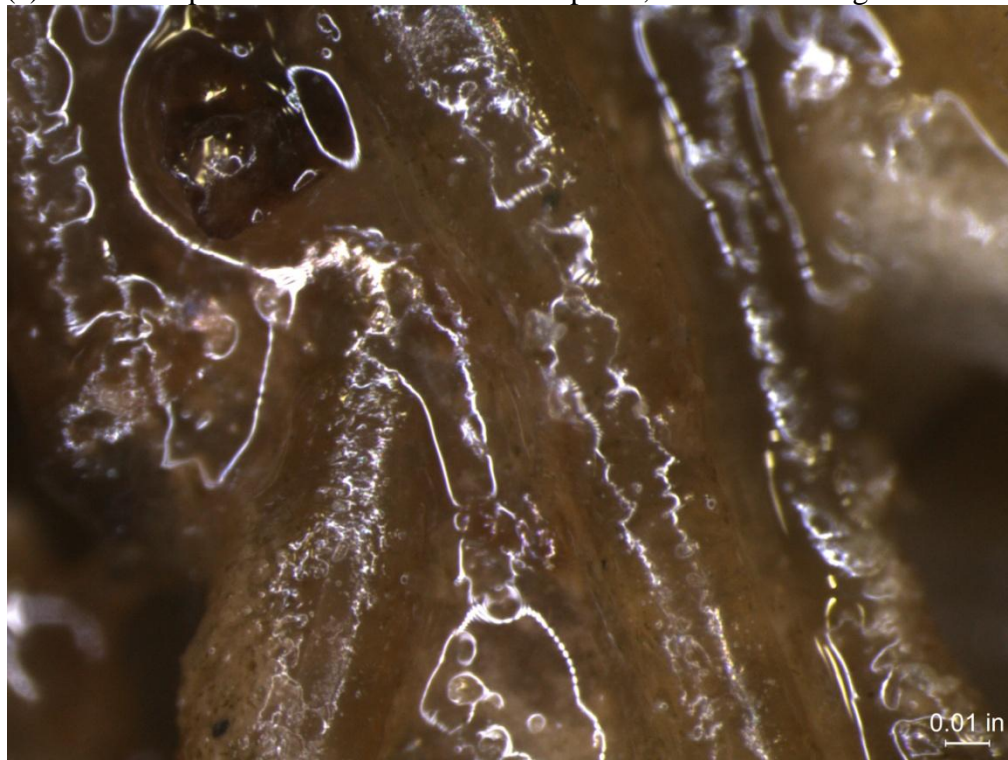
(b) Duplex 2205 Stainless Steel Coupon 8, Before Cleaning 50X
