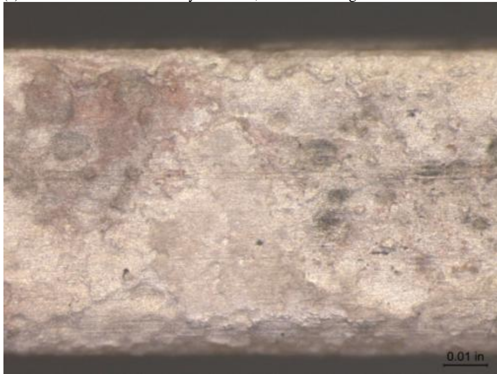
(b) Z-Alloy Screen 2, After Cleaning 50X
