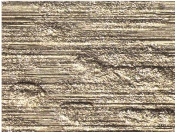
Photo 3-15. CDA 706 coupon 2 at 50x magnification after cleaning
