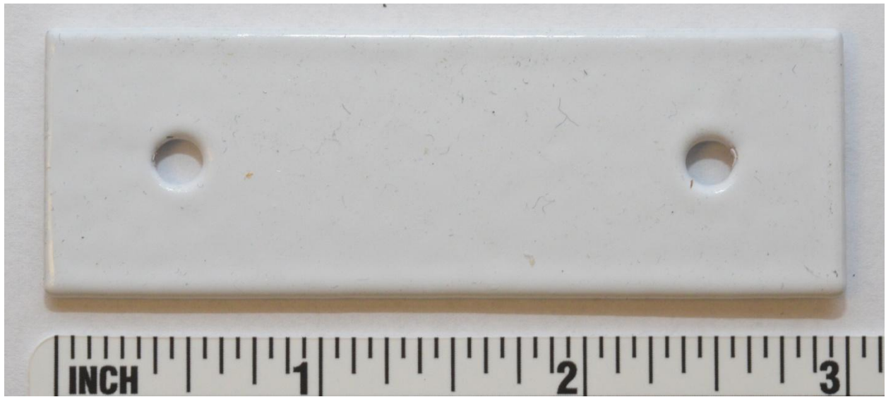
(a) Coated Duplex 2205 Stainless Steel Baseline Coupon, Front Side
