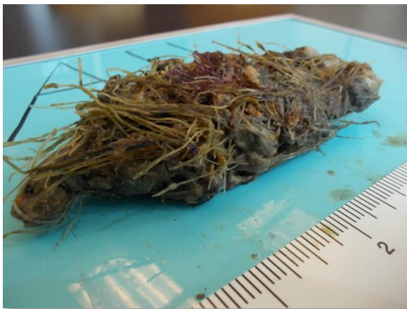
Photo 3-1. Marine life attached to uncoated 2205 Duplex stainless steel coupon with a weld.
