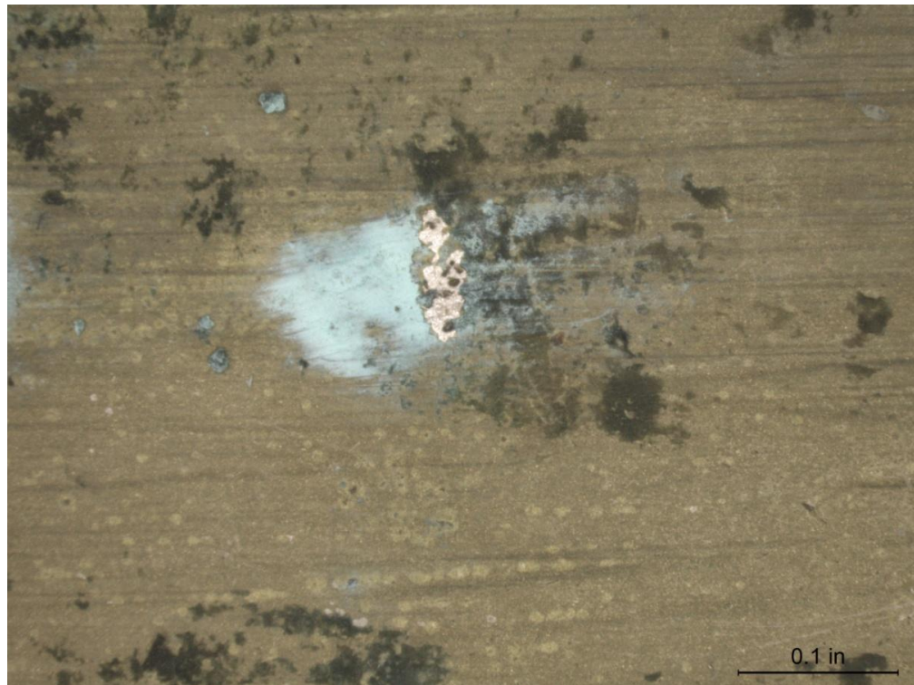
(a) Z-Alloy Coupon 4, Before Cleaning 10X
