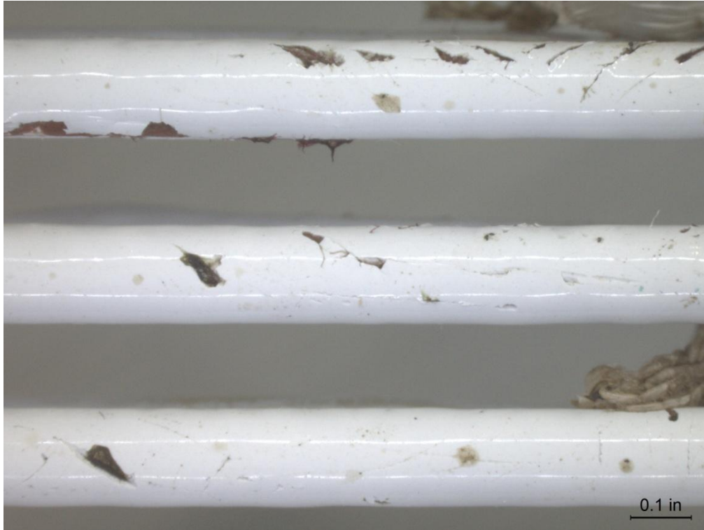
(a) Coated Duplex 2205 Stainless Steel Screen 3, Before Cleaning 10X
