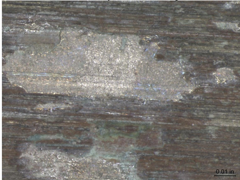
(b) CDA 715 Coupon 2, Before Cleaning 50X
