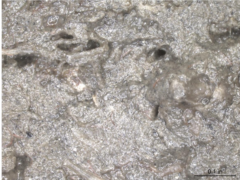
(a) Duplex 2205 Stainless Steel Screen 2, Before Cleaning 10X
