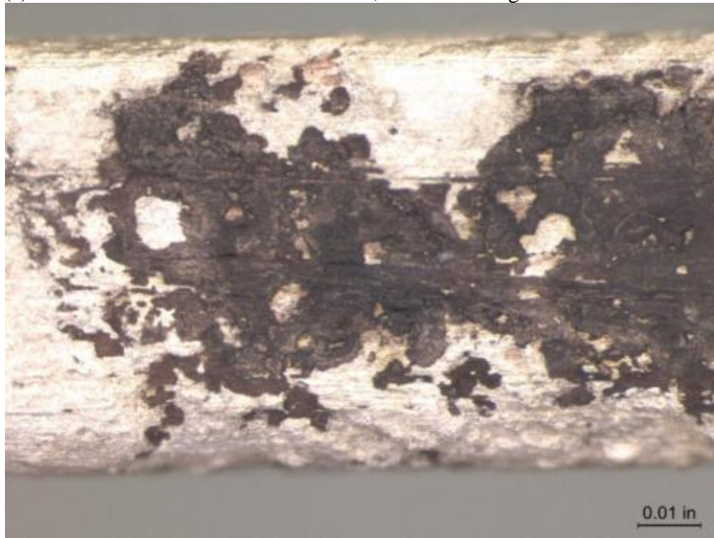
(b) CDA 706 Screen 2, After Cleaning 50X
