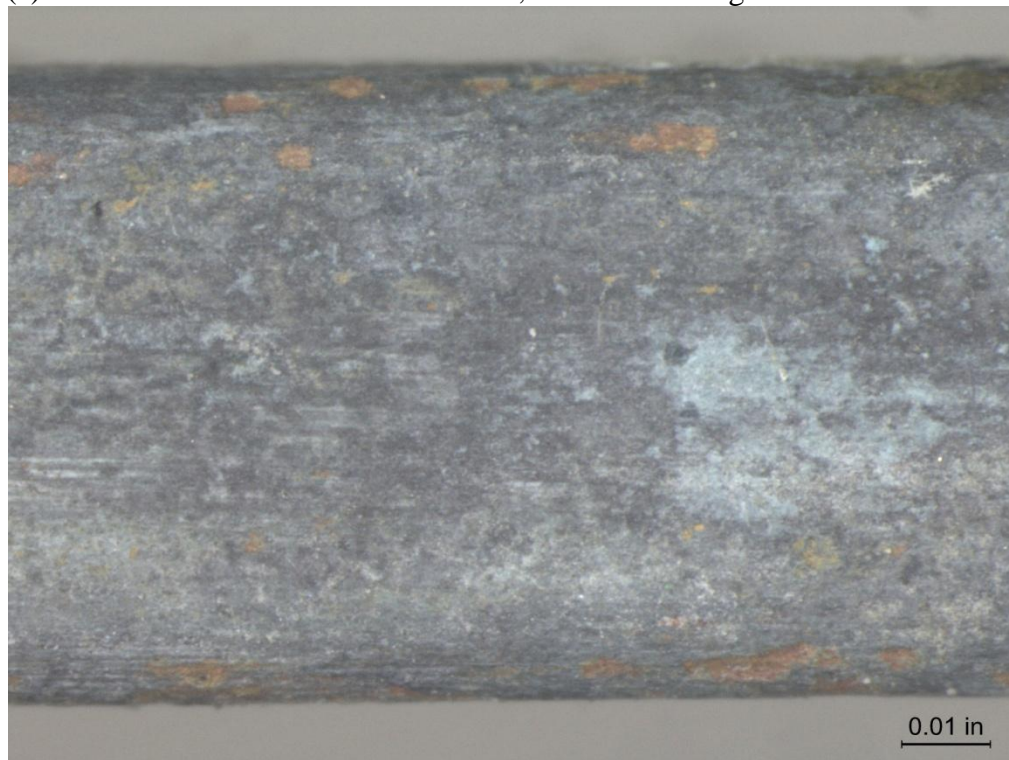
(b) CDA 706 Screen 2, Before Cleaning 50X
