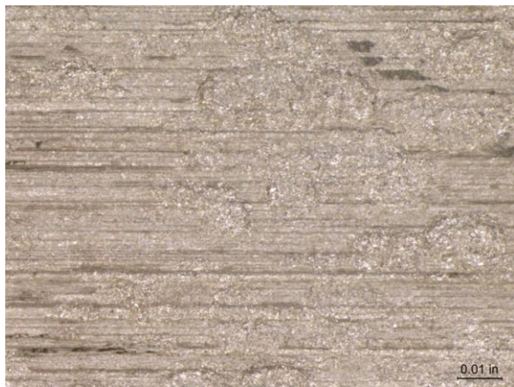
Photo 3-23. CDA 706 coupon at 50x magnification after cleaning.
