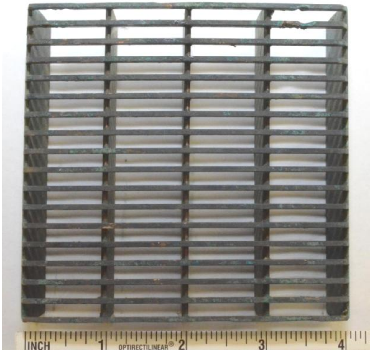
Figure 6 Photograph of CDA 706 screen 2 after a 6 month corrosion test.
