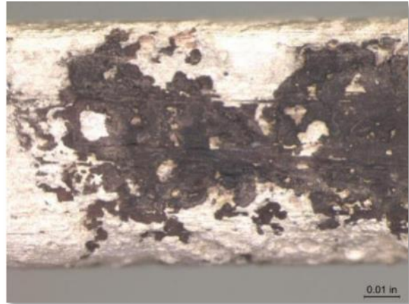
Photo 3-16. CDA 706 Screen 2 at 50X magnification after cleaning.
