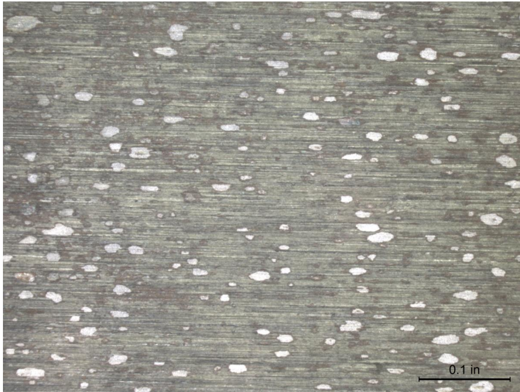
(a) CDA 715 Coupon 1, Before Cleaning 10X
