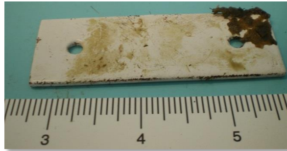
Photo 3-4. Slight damage to coating on edge and initiation of biofouling on corner of coated 2205 Duplex stainless steel coupon.
