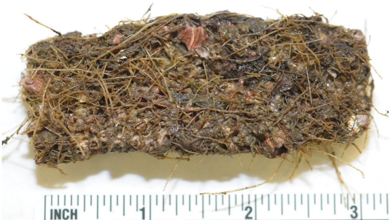
(a) Duplex 2205 Stainless Steel Coupon 6, Front Side
