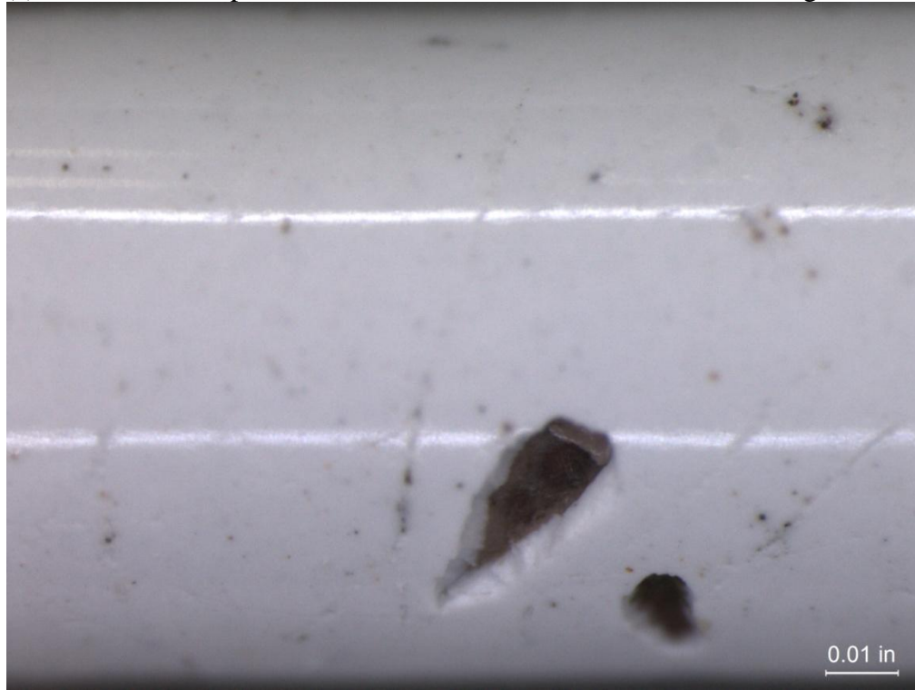
(b) Coated Duplex 2205 Stainless Steel Screen 3, After Cleaning 50X
