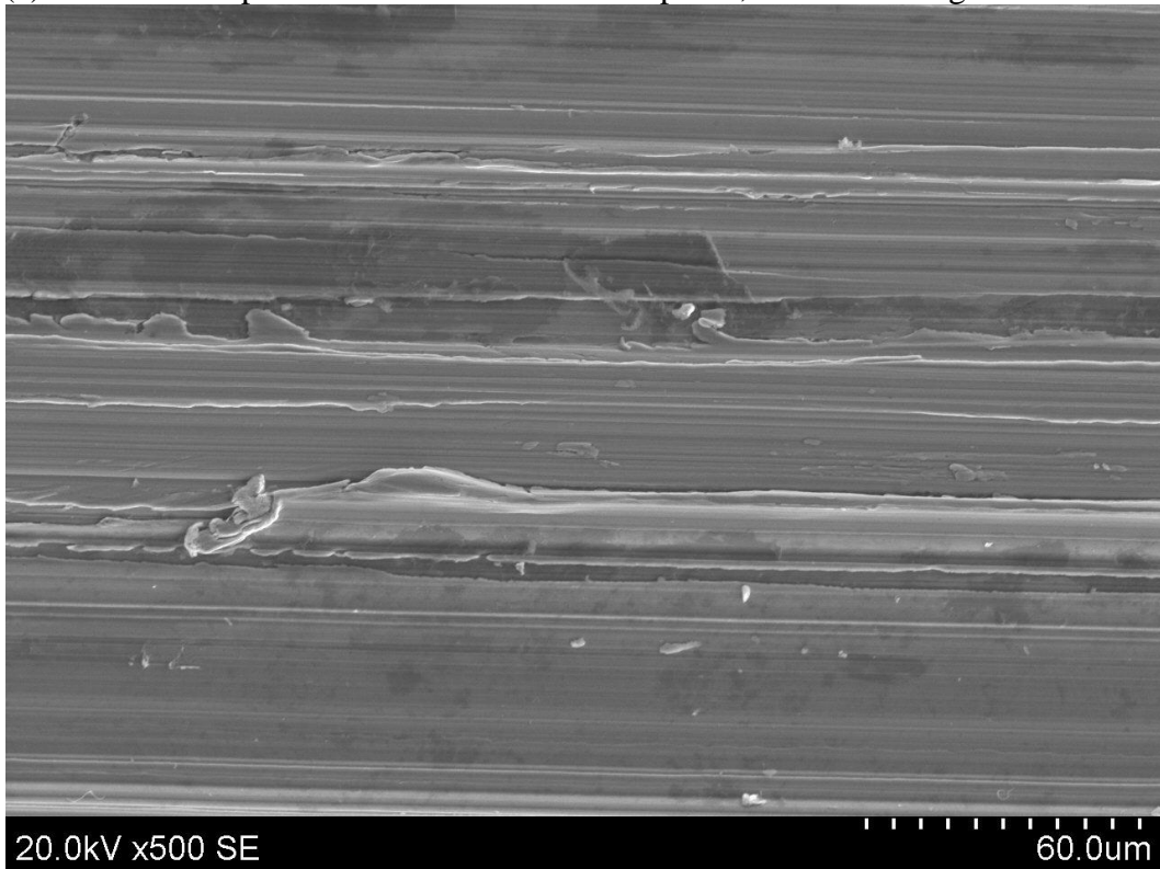
(b) Duplex 2205 Stainless Steel Coupon 9, After Cleaning 500X
