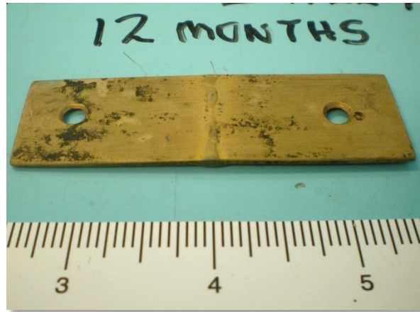
Photo 3-16. Z alloy 1-inch by 3-inch coupon with weld (front).
