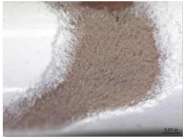
Photo 3-12. 2205 Duplex SS wedge wire screen surface at an area of coating damage.
