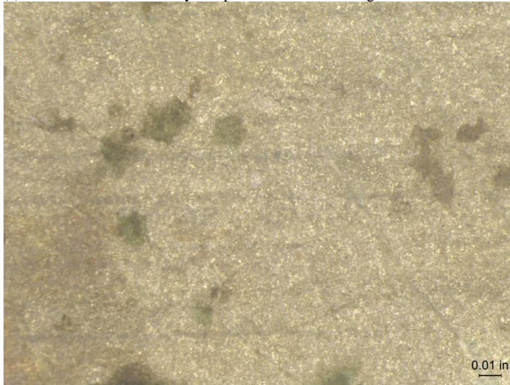
(b) Z-Alloy Coupon 3, Before Cleaning 50X
