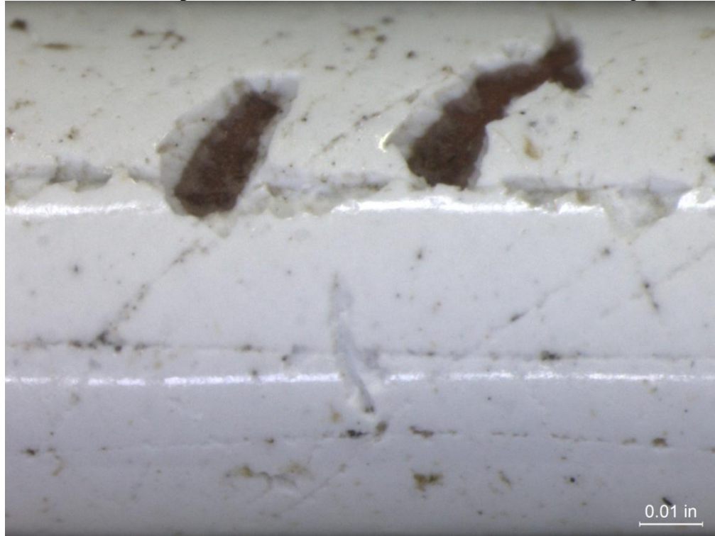
(b) Coated Duplex 2205 Stainless Steel Screen 4, After Cleaning 50X
