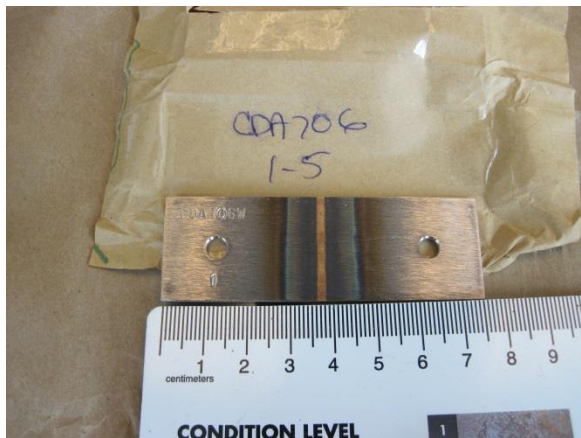
Photo 2-9. 90-10 Cu-Ni 1-inch by 3-inch coupon with weld
