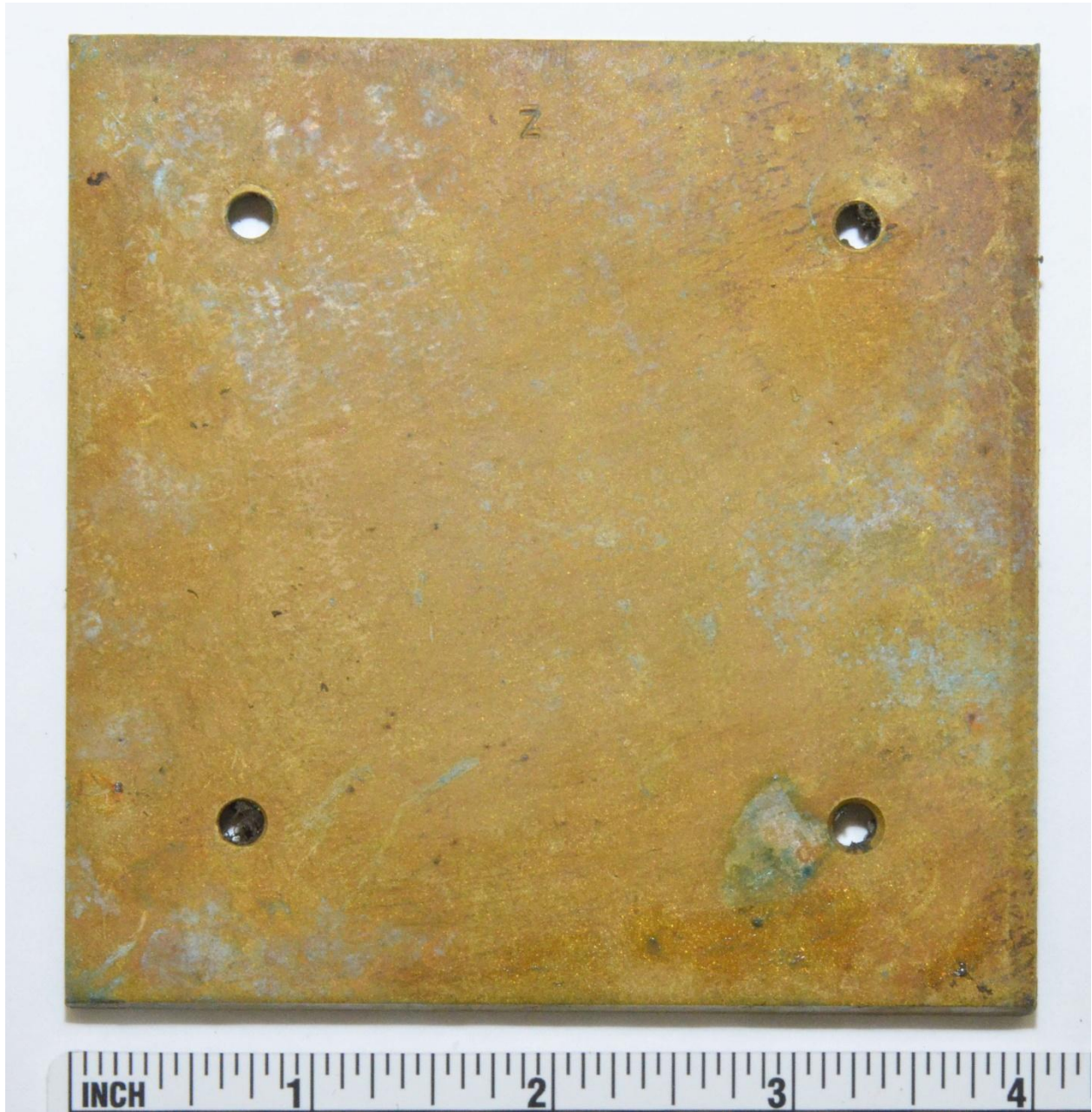
Figure 12 Photograph of the Z- Alloy plate after a 12 month corrosion test.
