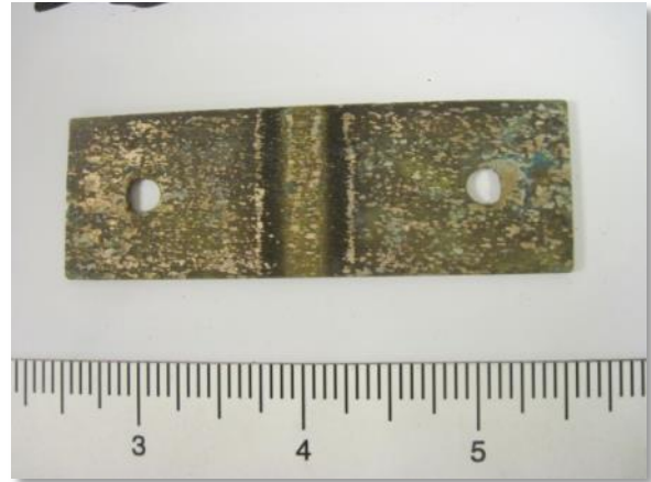
Photo 3-6. 90-10 Cu-Ni 1-inch by 3-inch coupon with weld
