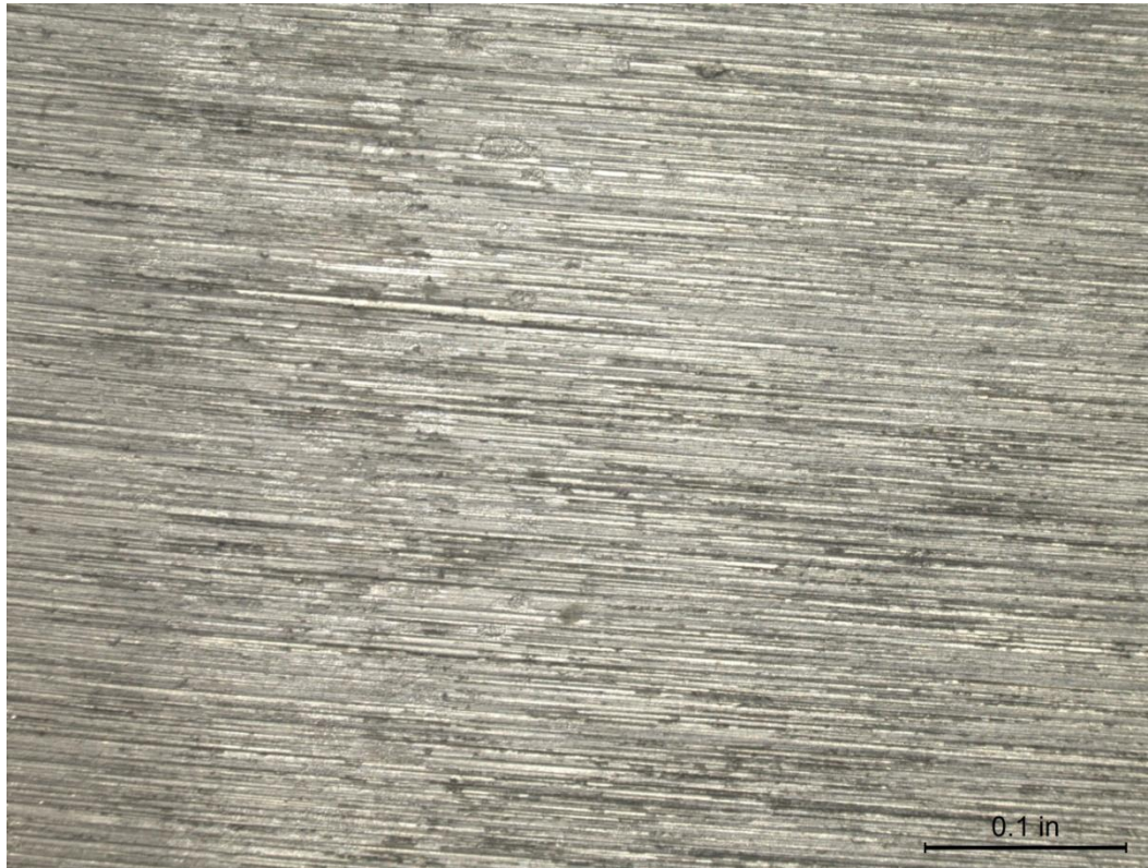
(a) CDA 715 Coupon 1, After Cleaning 10X
