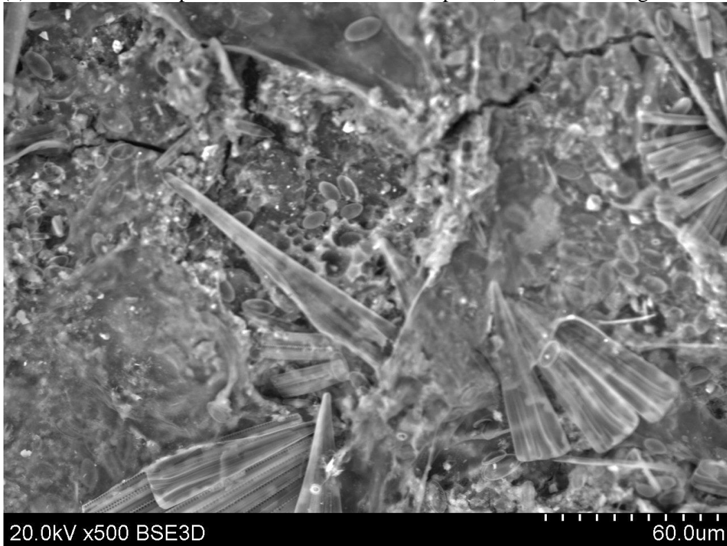
(b) Coated Duplex 2205 Stainless Steel Coupon 3, Before Cleaning 500X
