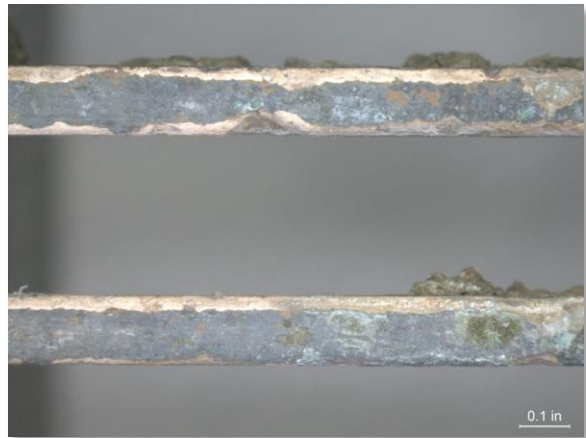
Photo 3-10. Mechanical damage to 90-10 Cu-Ni wedge wire screen.
