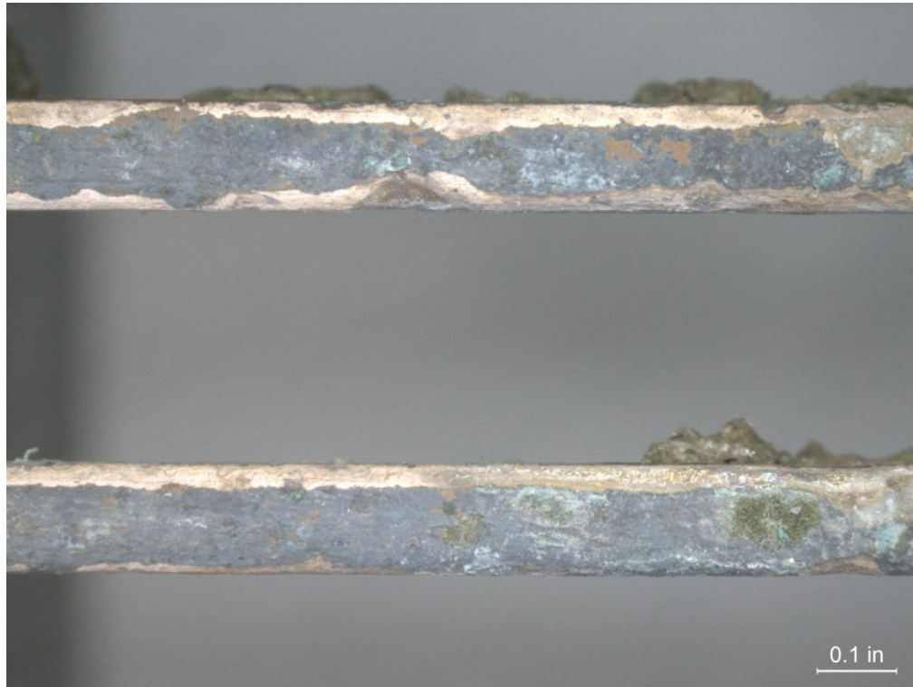
(a) CDA 706 Screen 3, Before Cleaning 10X
