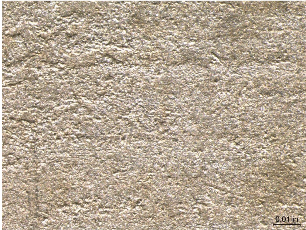
(b) Z-Alloy Coupon 2, After Cleaning 50X
