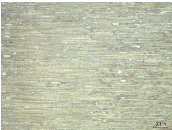
Photo 3-7. 70-30 Cu-Ni coupon at 10x magnification.
