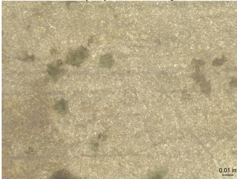
(b) Z-Alloy Coupon 3, Before Cleaning 50X
