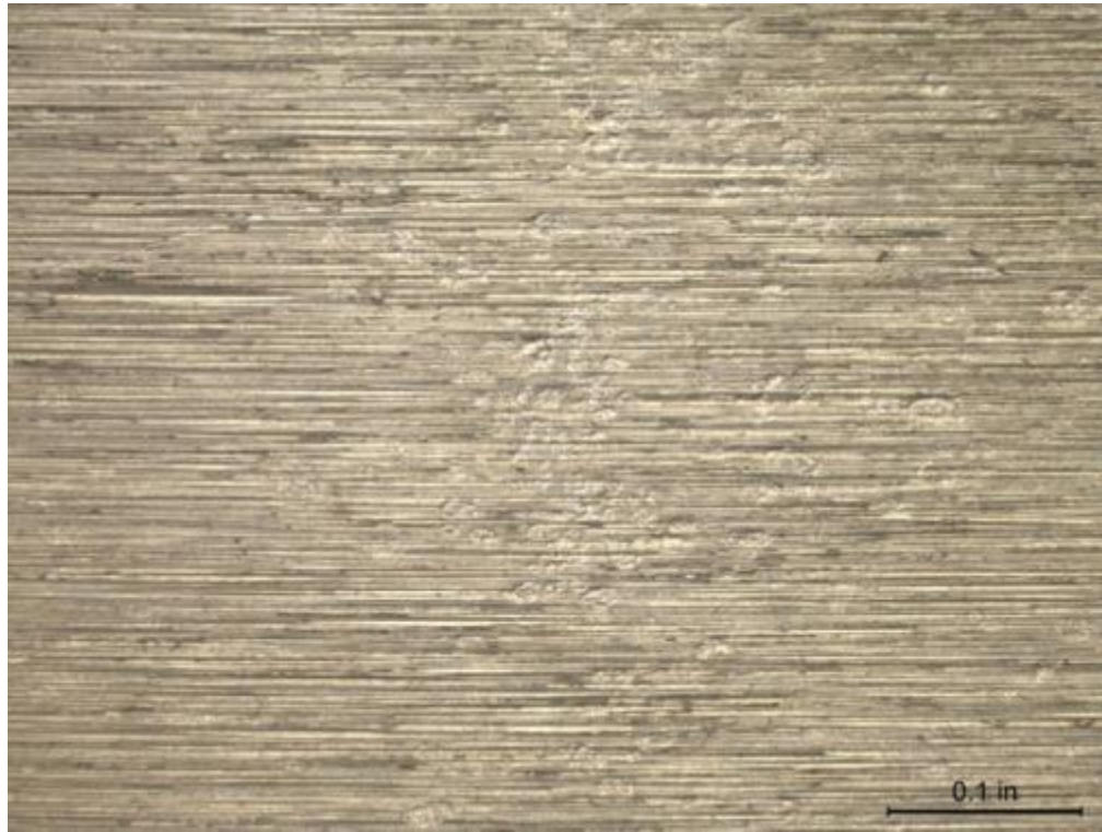
(a) CDA 706 Coupon 1, After Cleaning 10X
