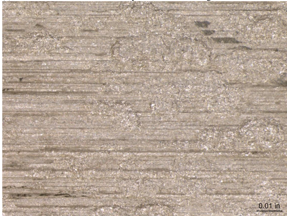
(b) CDA 706 Coupon 3, After Cleaning 50X
