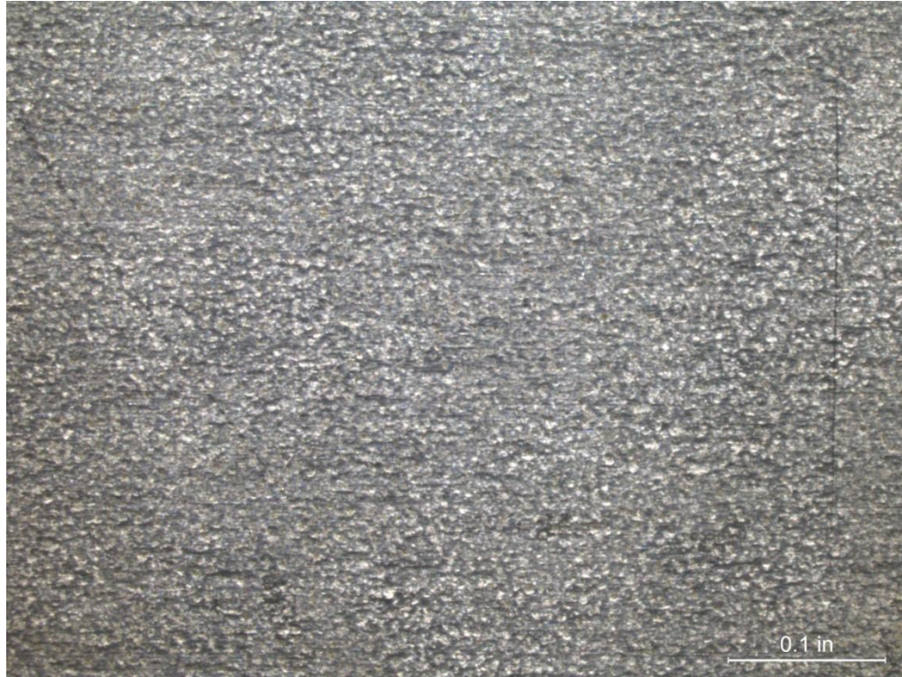
(a) Duplex 2205 Stainless Steel Plate, After Cleaning 10X
