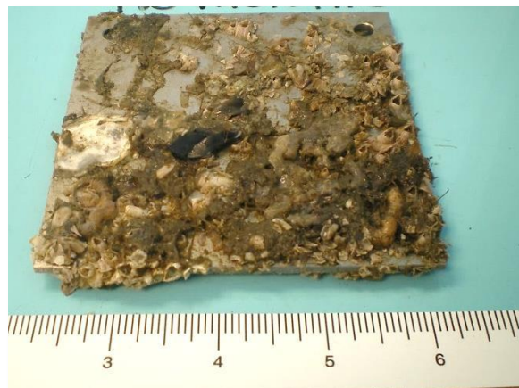
Photo 3-2. Marine life attached to uncoated 2205 Duplex stainless steel flat plate.
