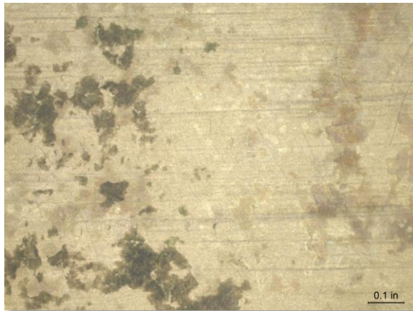
Photo 3-15. Z alloy coupon at 10x magnification.
