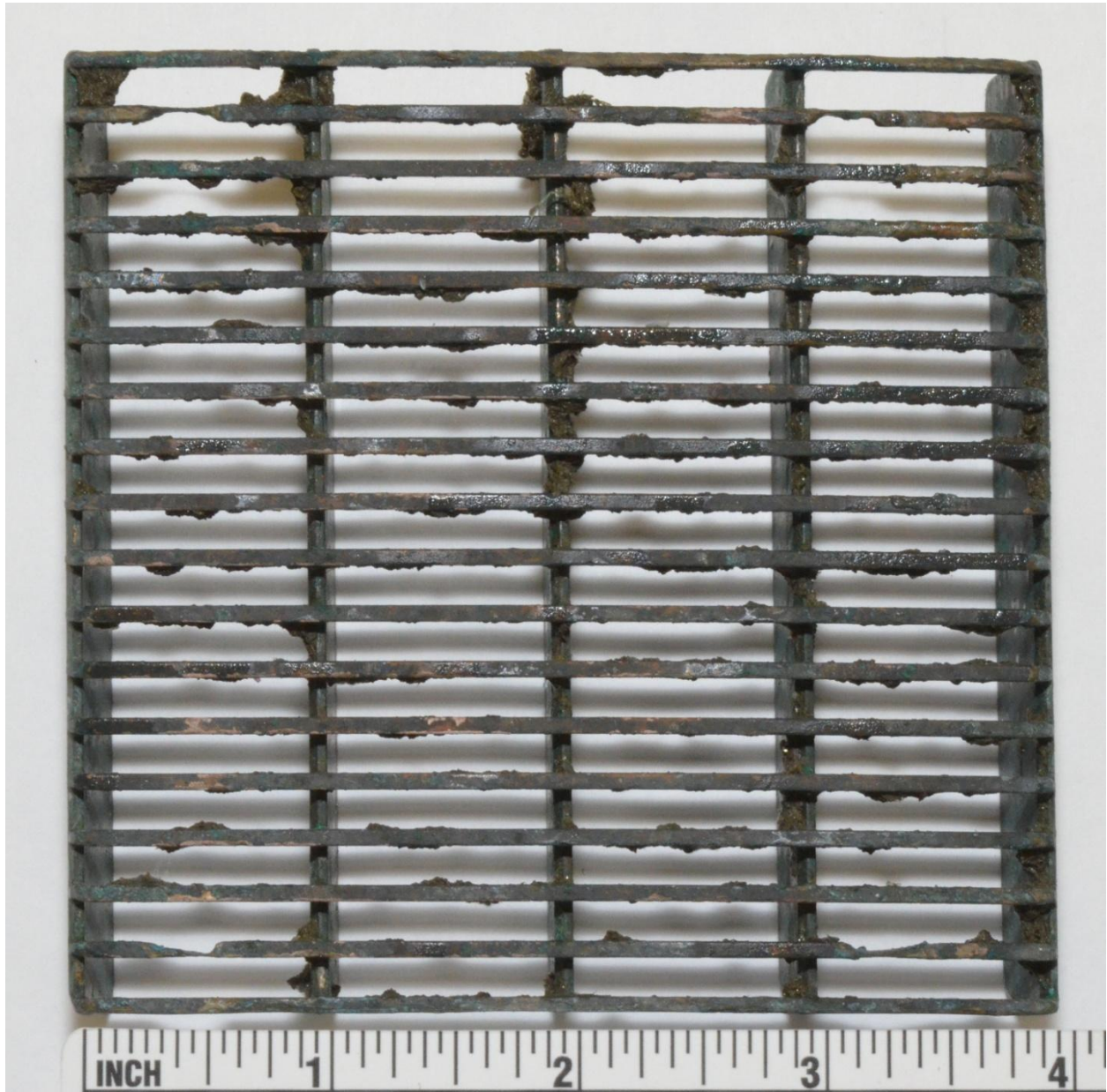
Figure 10 Photograph of CDA 706 screen 4 after a 12 month corrosion test.
