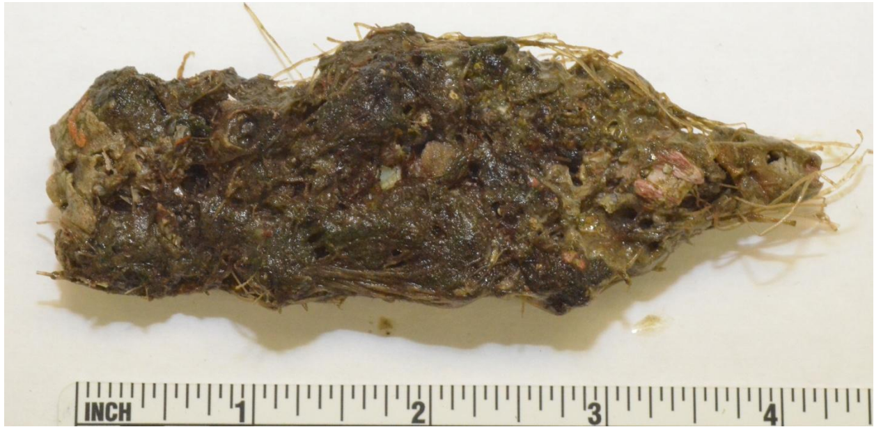
(a) Duplex 2205 Stainless Steel Coupon 8, Front Side
