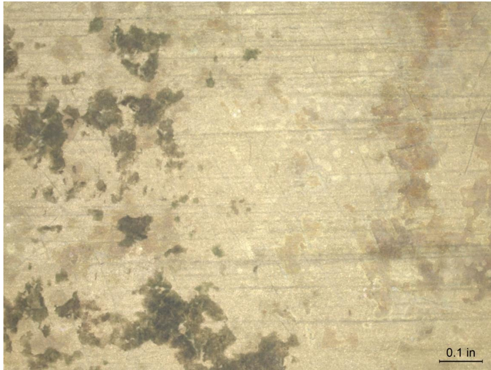
(a) Z-Alloy Coupon 3, Before Cleaning 10X
