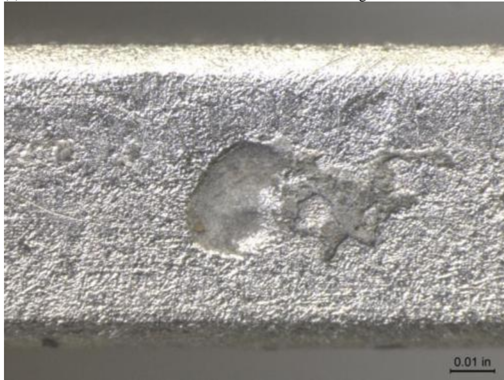
(b) CDA 715 Screen 1, After Cleaning 50X
