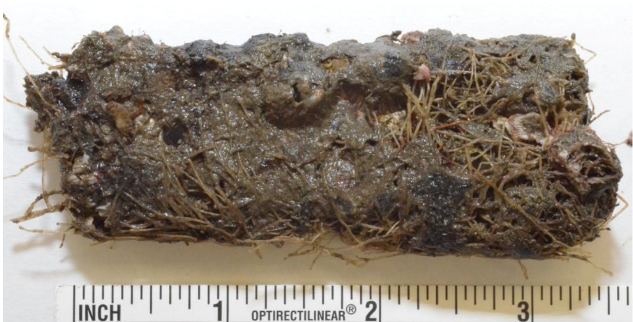
(b) Duplex 2205 Stainless Steel Coupon 7, Back Side
