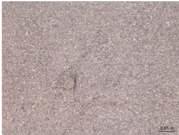
Photo 3-25. Z Alloy coupon at 50X magnification after cleaning.
