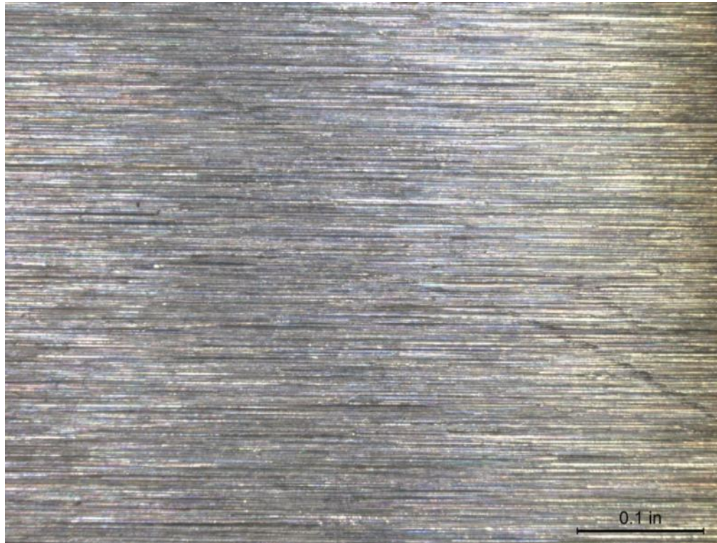
(a) Duplex 2205 Stainless Steel Coupon 6, After Cleaning 10X
