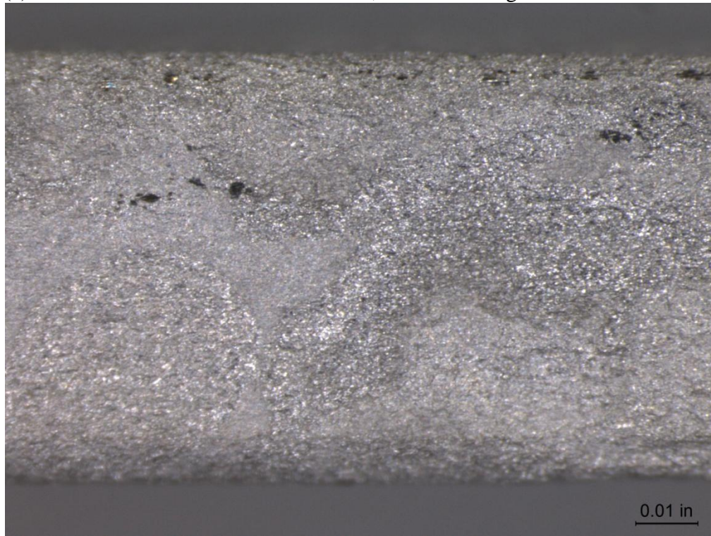
(b) CDA 715 Screen 3, After Cleaning 50X
