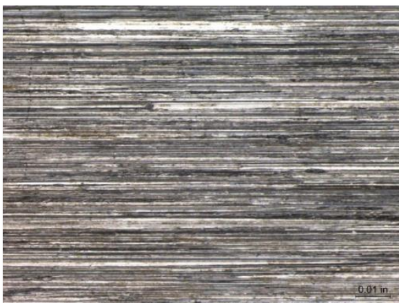
Photo 3-11. 2205 Duplex SS coupon surface exposed at an area of coating damage.
