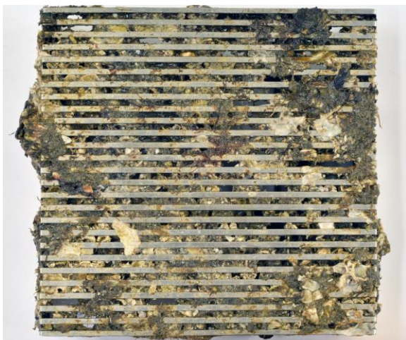
Photo 3-1. Uncoated 2205 Duplex SS wedge wire screen, before cleaning.
