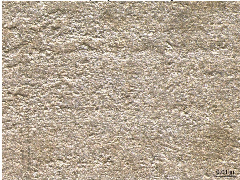
(b) Z-Alloy Coupon 2, After Cleaning 50X
