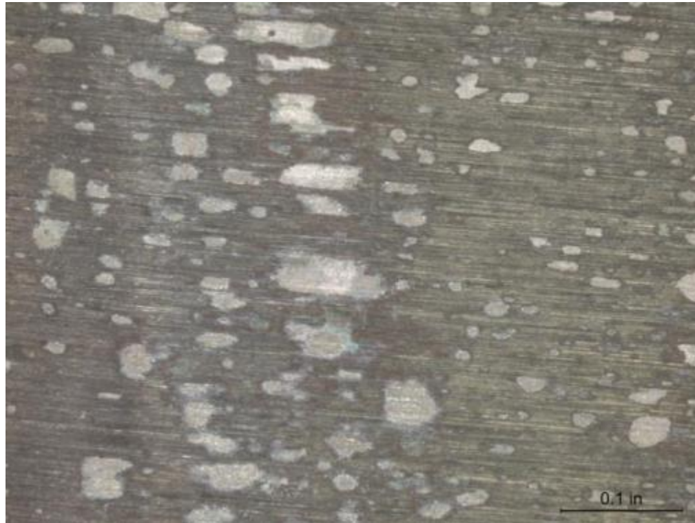
(a) CDA 715 Coupon 2, Before Cleaning 10X
