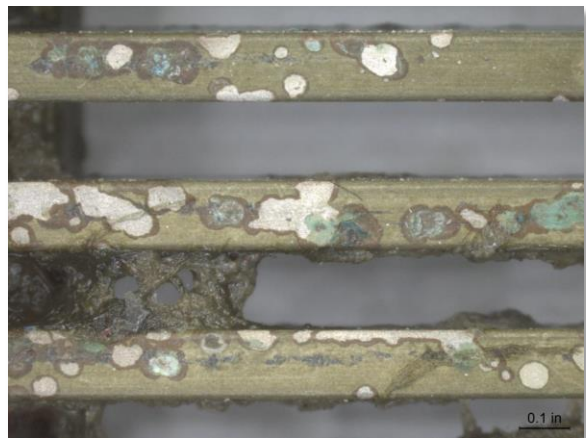
Photo 3-8. 70-30 Cu-Ni wire screen at 10x magnification.
