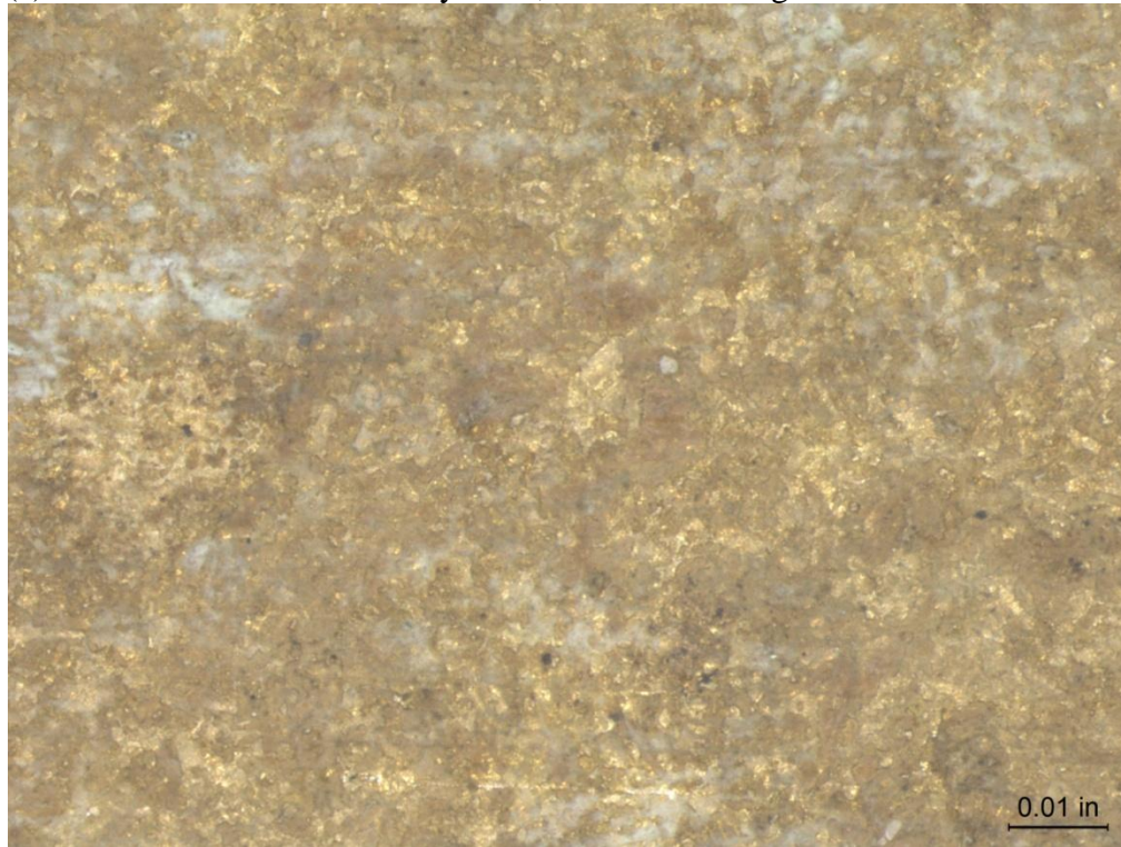
(b) Z-Alloy Plate, Before Cleaning 50X
