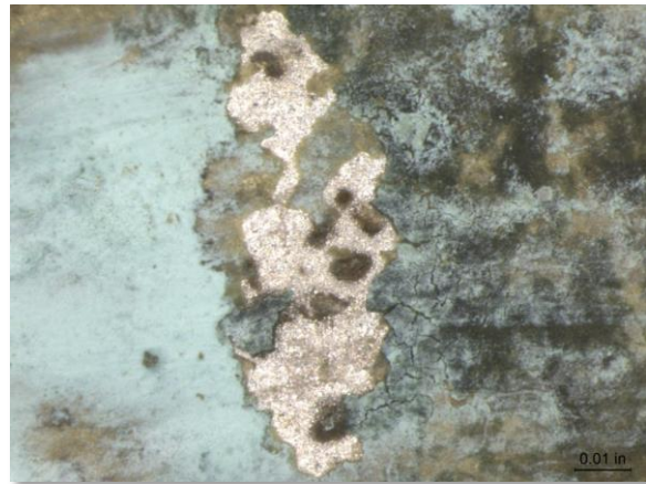
Photo 3-18. Surface discoloration of Z alloy coupon, shown at 50x magnification
