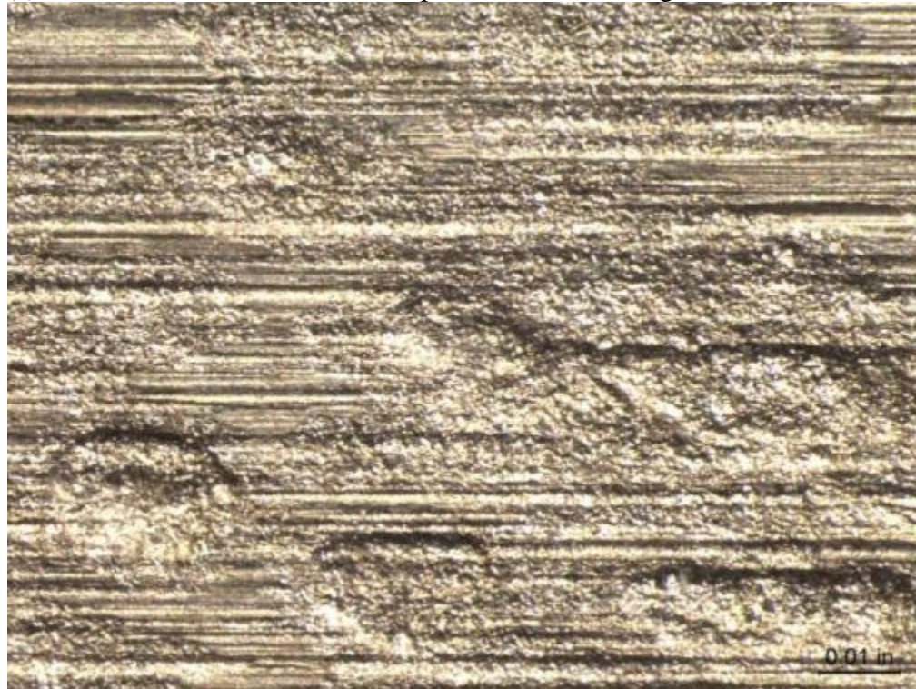
(b) CDA 706 Coupon 2, After Cleaning 50X
