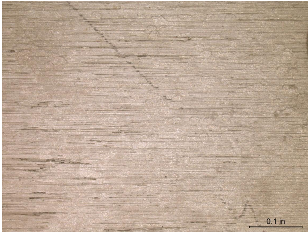
(a) CDA 706 Coupon 3, After Cleaning 10X
