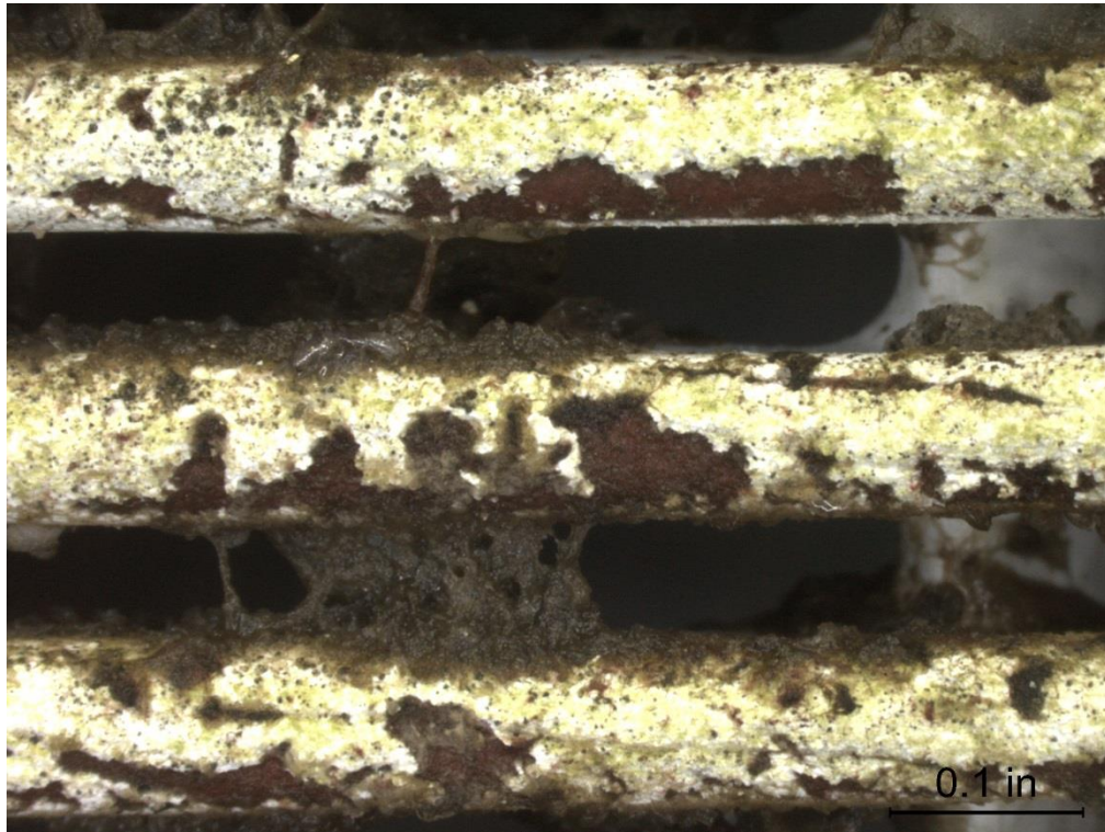
(a) Coated Duplex 2205 Stainless Steel Screen 5, Before Cleaning 10X
