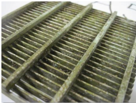
Photo 3-3. 70-30 Cu-Ni 4-inch by 4-inch wedge wire screen
