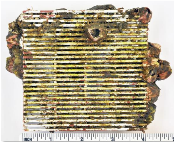
Photo 3-5. Coated 2205 Duplex SS wire screen, before cleaning.
