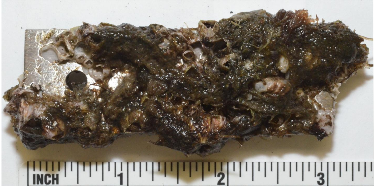
(a) Duplex 2205 Stainless Steel Coupon 9, Front Side
