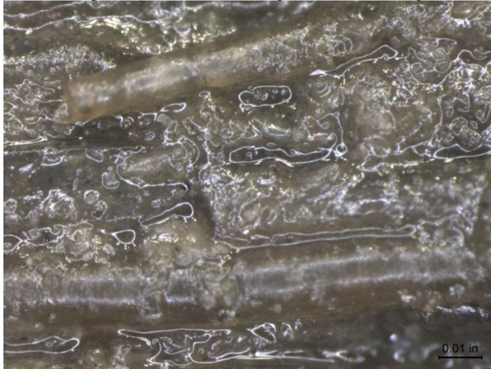
(b) Duplex 2205 Stainless Steel Coupon 6, Before Cleaning 50X
