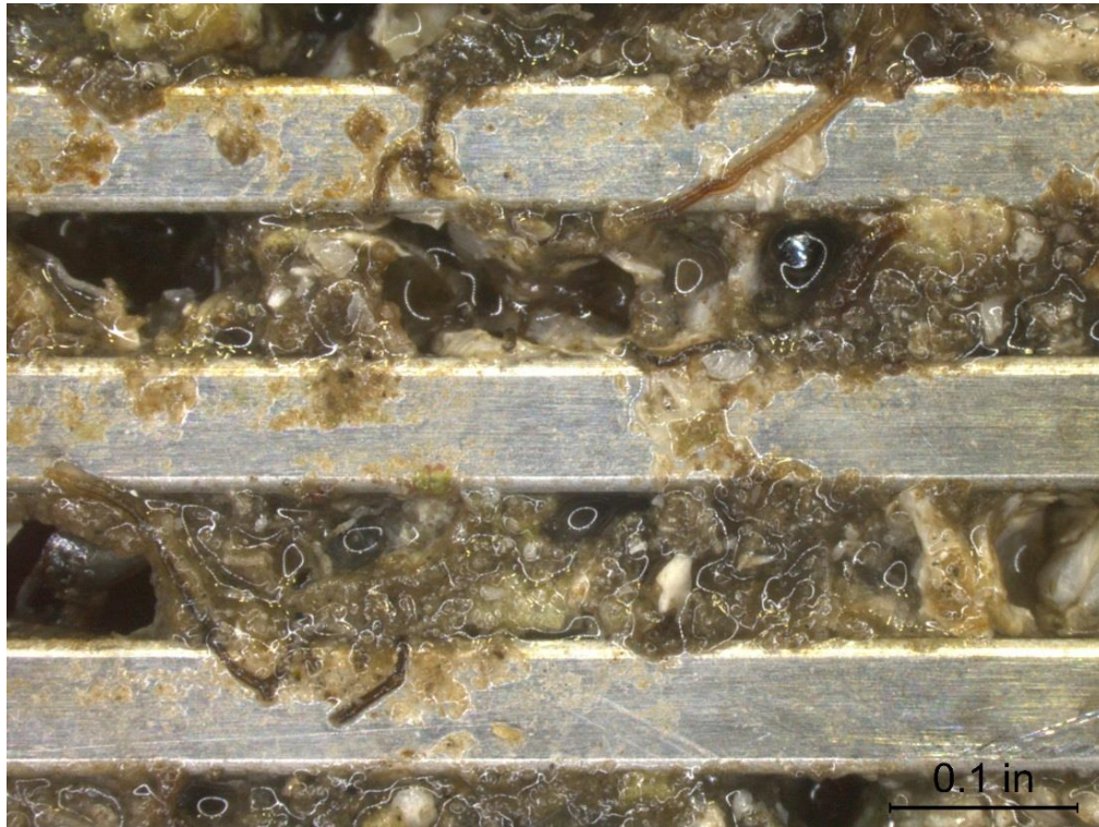
(a) Duplex 2205 Stainless Steel Screen 5, Before Cleaning 10X
