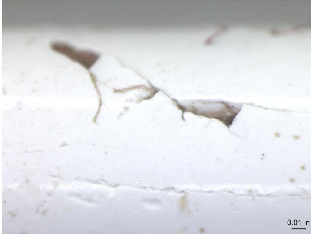
(b) Coated Duplex 2205 Stainless Steel Screen 3, Before Cleaning 50X
