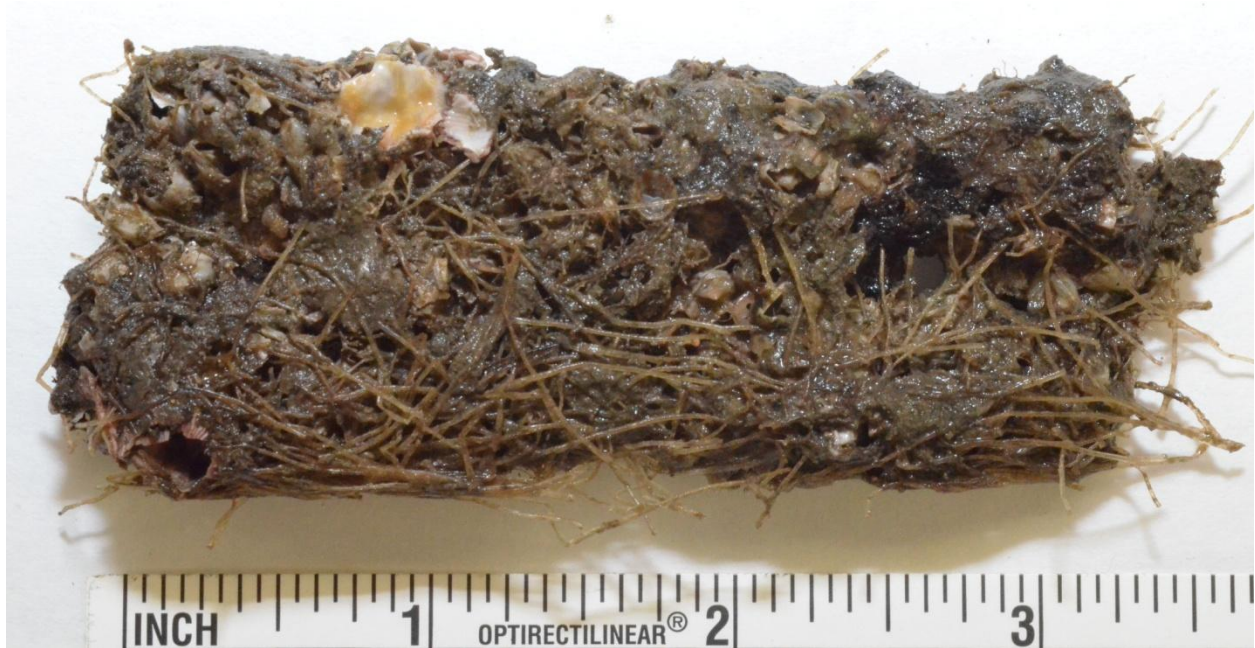
(a) Duplex 2205 Stainless Steel Coupon 7, Front Side
