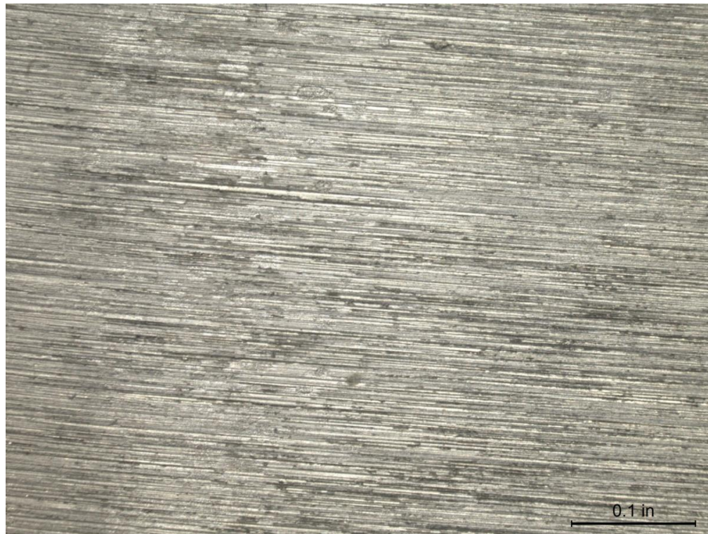
(a) CDA 715 Coupon 1, After Cleaning 10X
