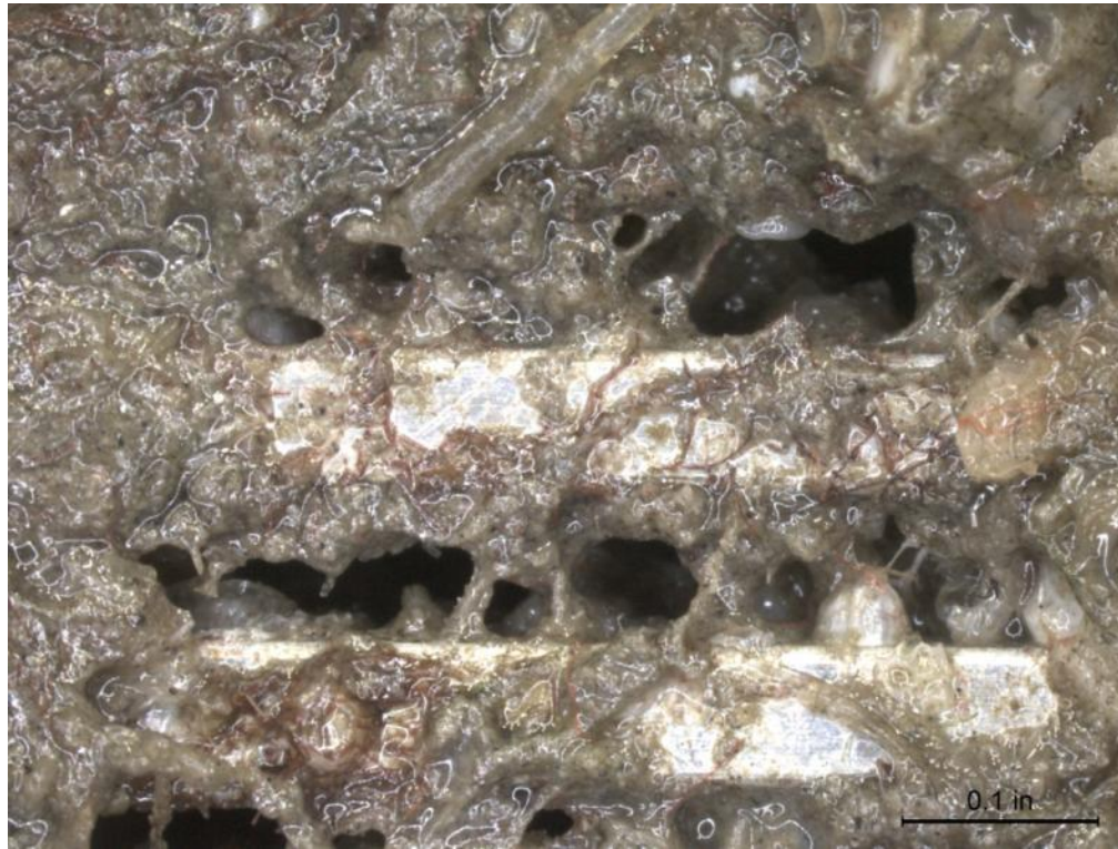
(a) Duplex 2205 Stainless Steel Screen 1, Before Cleaning 10X
