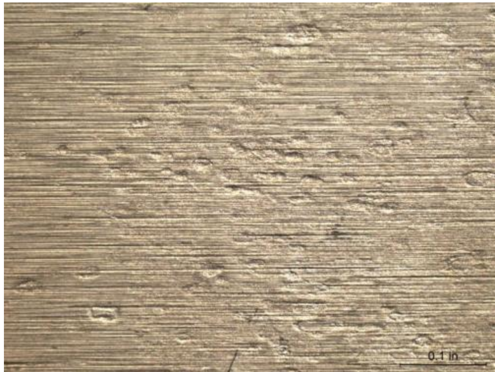
(a) CDA 706 Coupon 2, After Cleaning 10X
