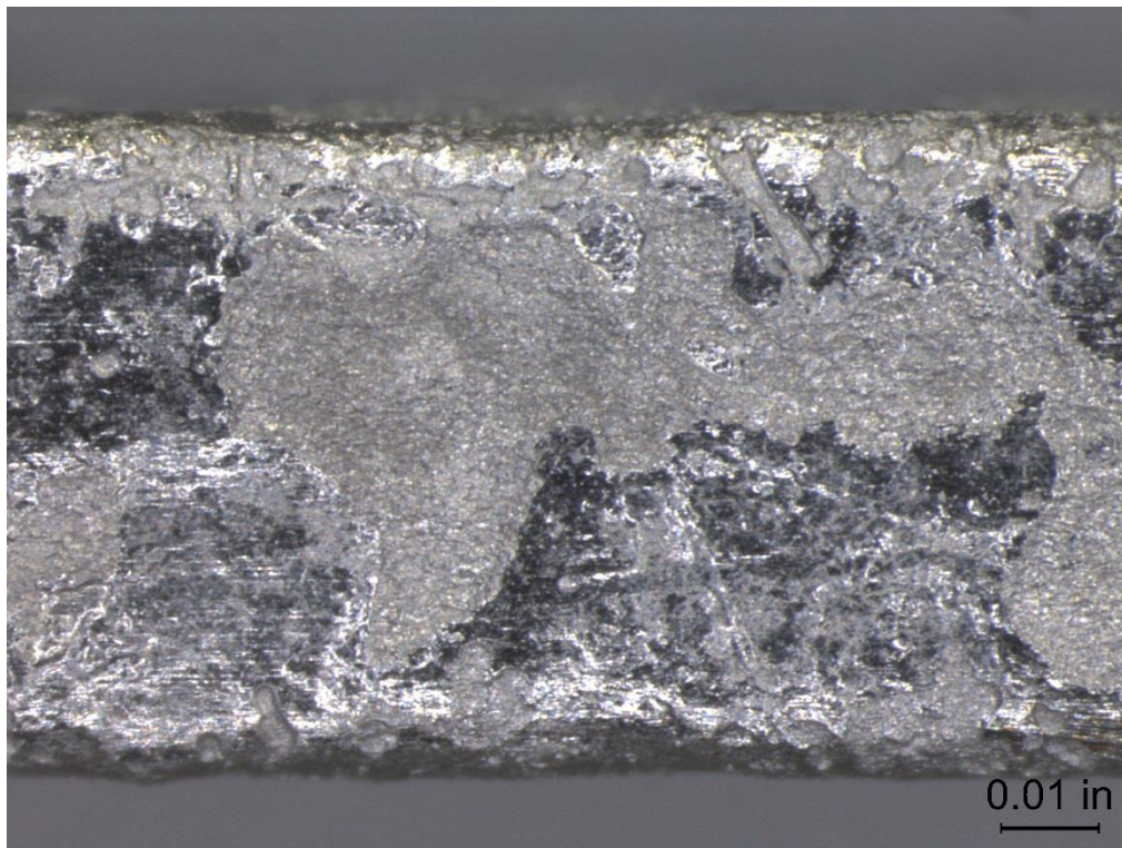
(b) CDA 715 Screen 5, After Cleaning 50X
