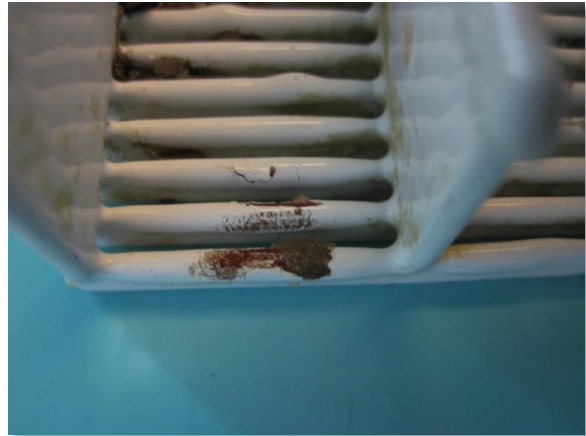
Photo 3-4. Coating damage to 2205 Duplex Stainless Steel wedge wire sample.
