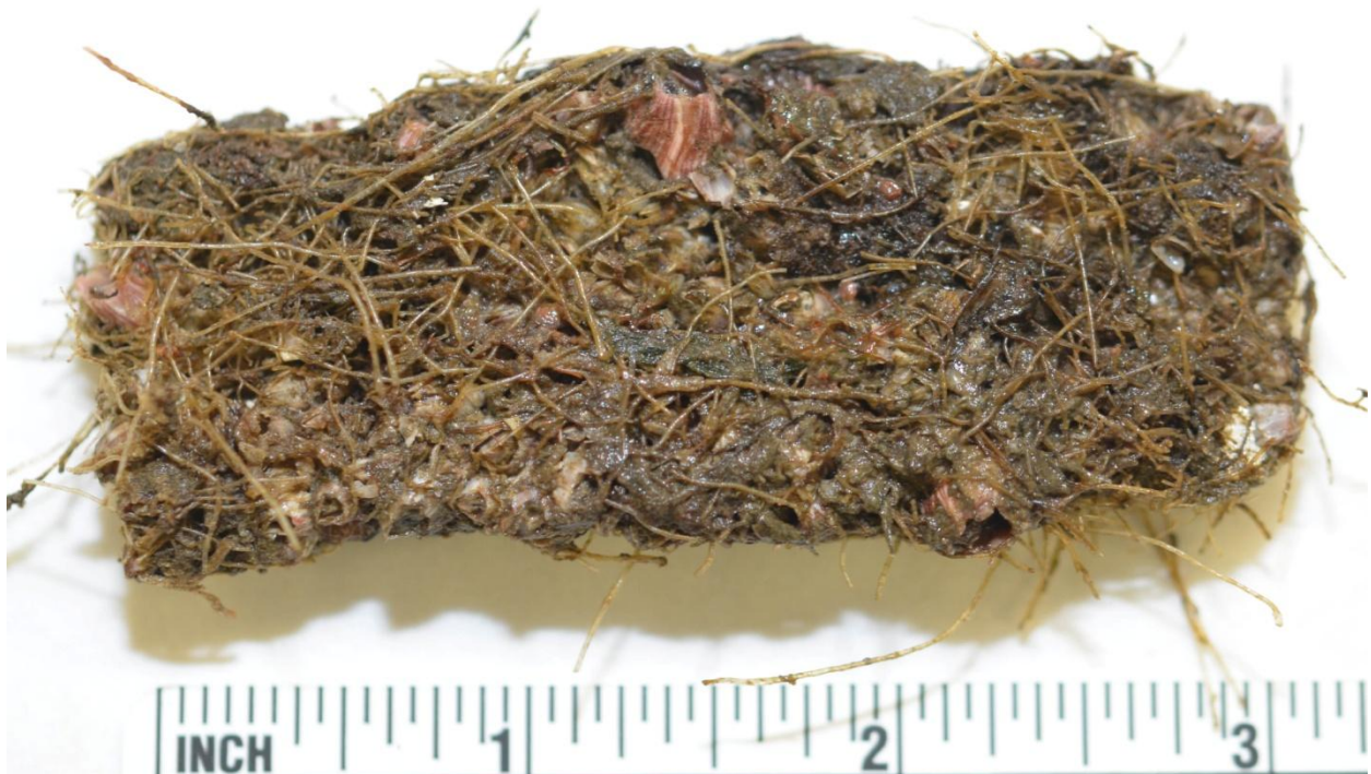
(a) Duplex 2205 Stainless Steel Coupon 6, Front Side
