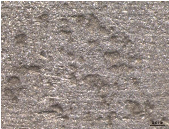
Photo 3-33. Z Alloy coupon at 50X magnification after cleaning.
