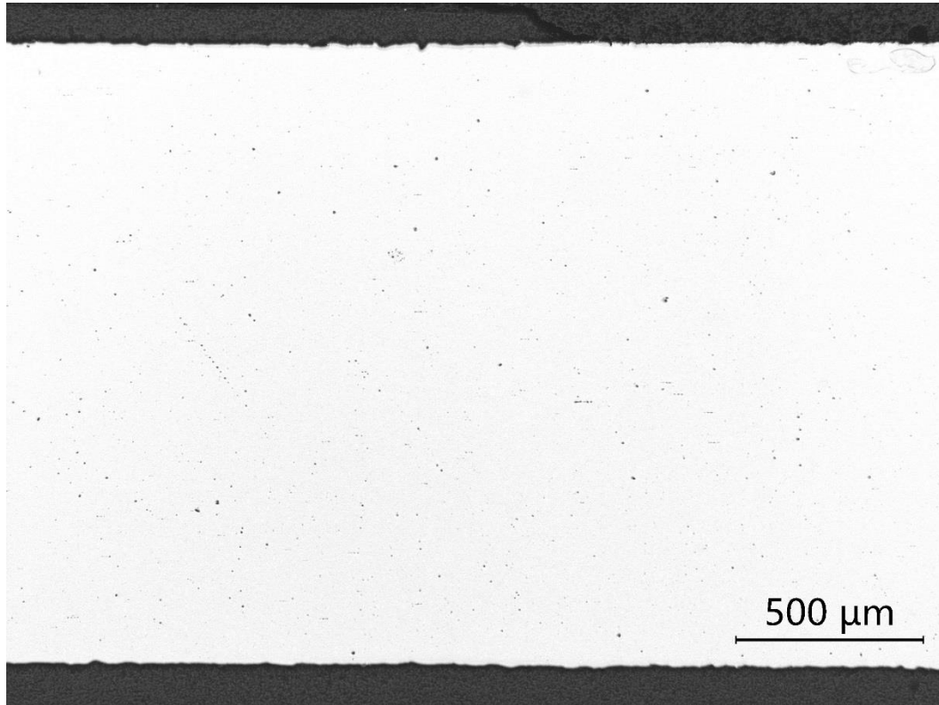
(a) Coated Duplex 2205 Stainless Steel Screen 5 50X
