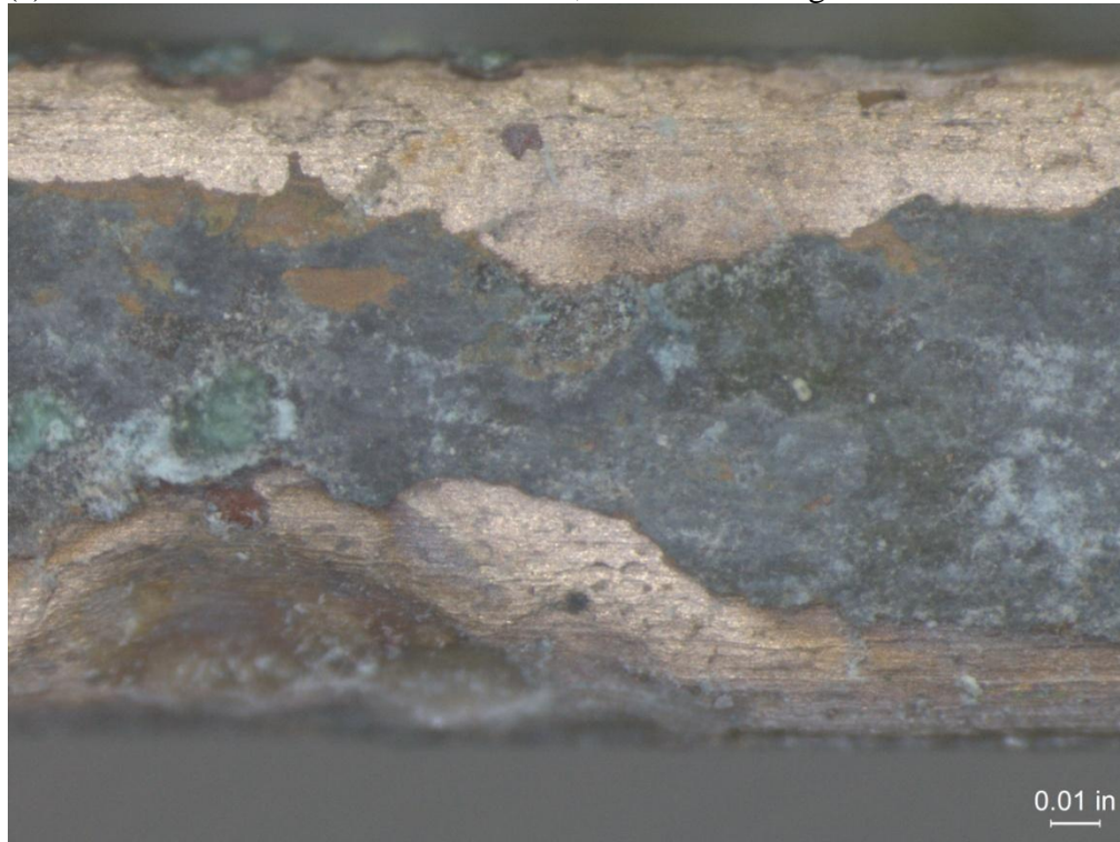
(b) CDA 706 Screen 3, Before Cleaning 50X
