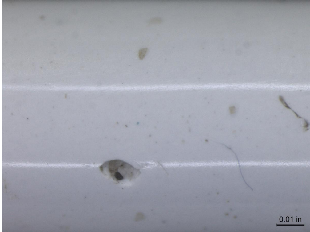
(b) Coated Duplex 2205 Stainless Steel Screen 1, Before Cleaning 50X
