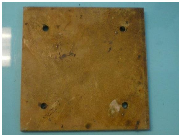
Photo 3-19. Minimal corrosion was observed on the Z alloy flat plate.
