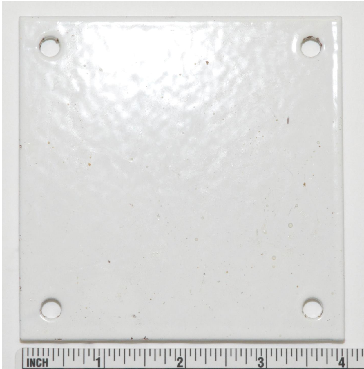
(a) Coated Duplex 2205 Stainless Steel Plate
