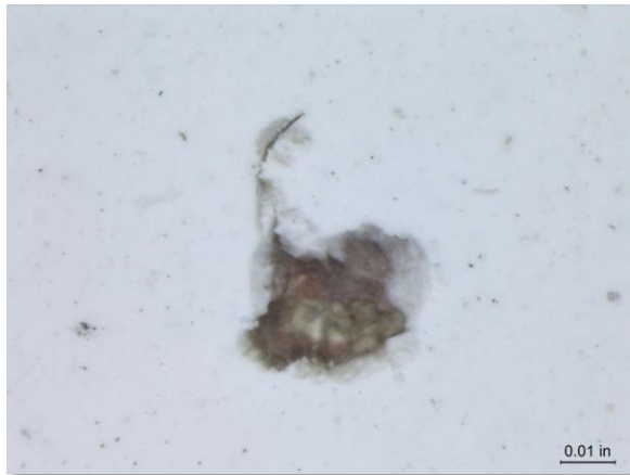
Photo 3-19. 2205 Duplex SS coupon surface exposed at an area of coating damage.
