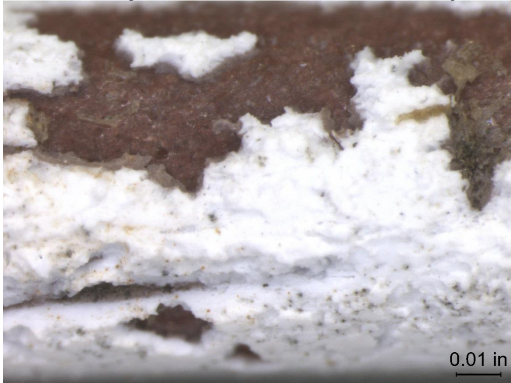
(b) Coated Duplex 2205 Stainless Steel Screen 5, After Cleaning 50X
