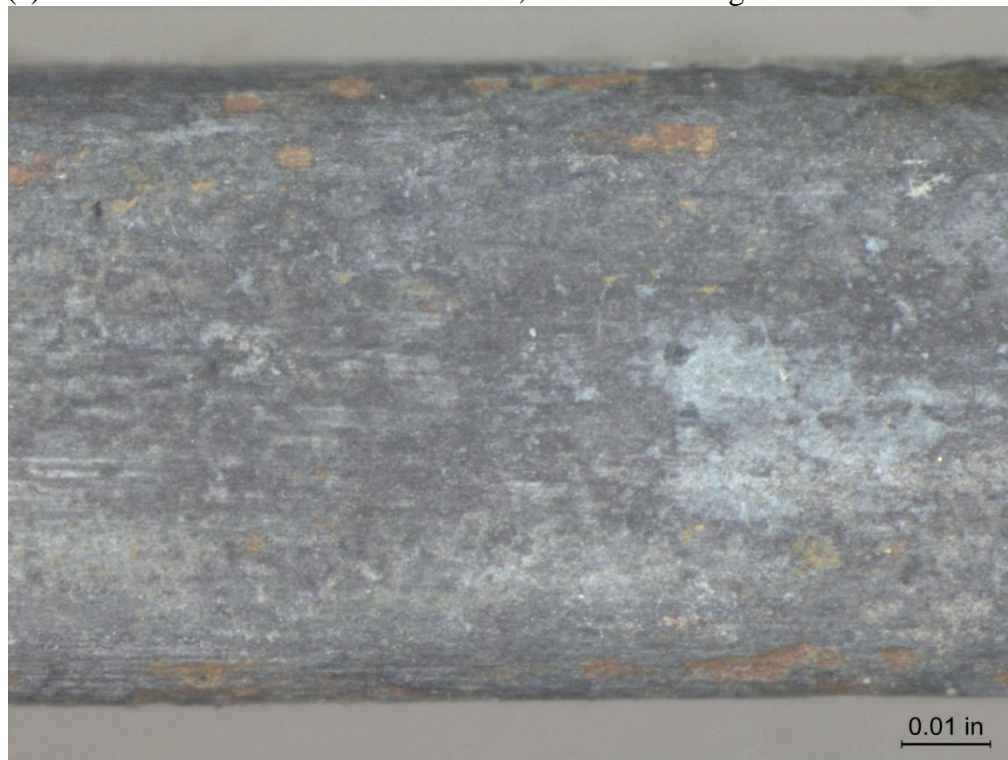
(b) CDA 706 Screen 2, Before Cleaning 50X
