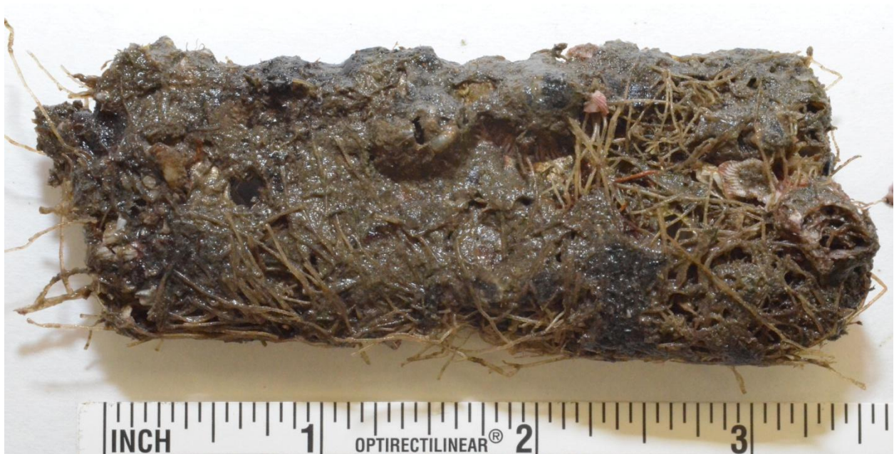
(b) Duplex 2205 Stainless Steel Coupon 7, Back Side
