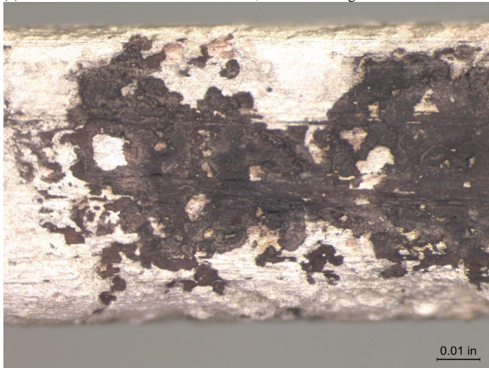
(b) CDA 706 Screen 2, After Cleaning 50X
