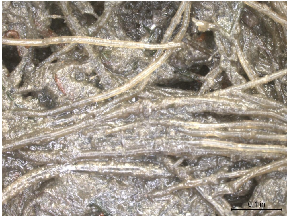
(a) Duplex 2205 Stainless Steel Coupon 6, Before Cleaning 10X
