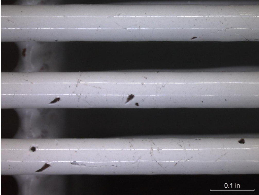
(a) Coated Duplex 2205 Stainless Steel Screen 3, After Cleaning 10X
