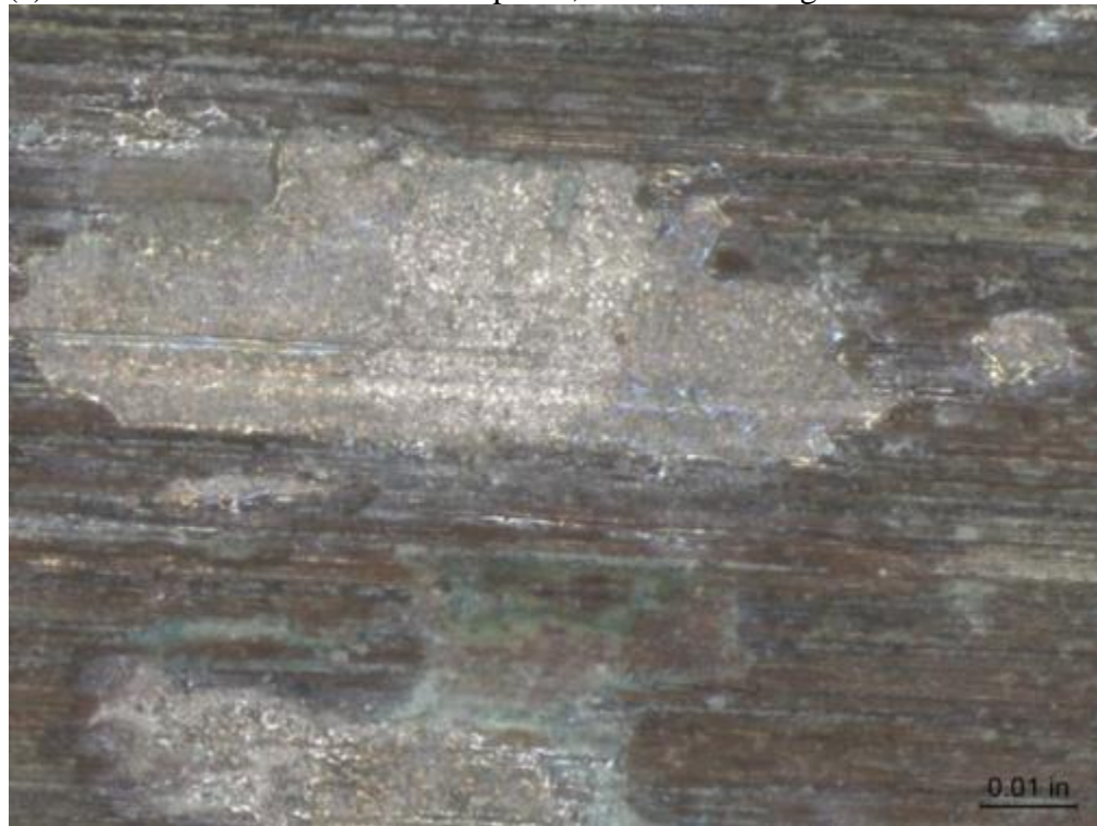
(b) CDA 715 Coupon 2, Before Cleaning 50X
