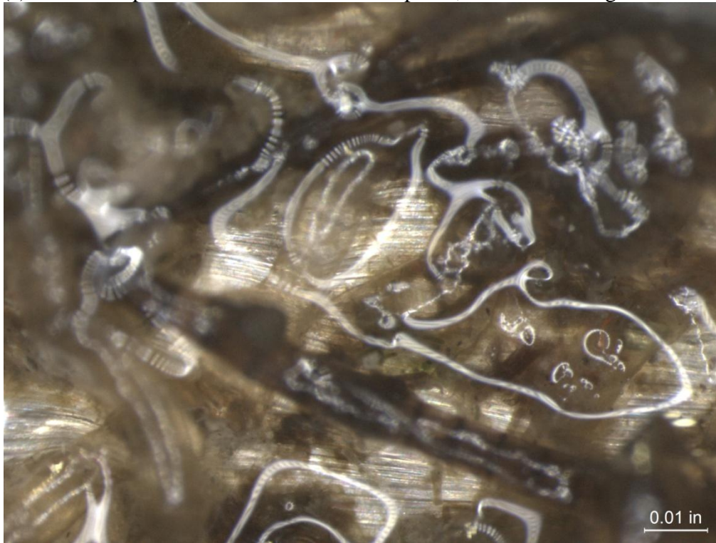
(b) Duplex 2205 Stainless Steel Coupon 9, Before Cleaning 50X
