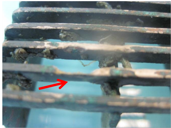
Photo 3-10. Mechanical damage to 90-10 Cu-Ni wedge wire screen.
