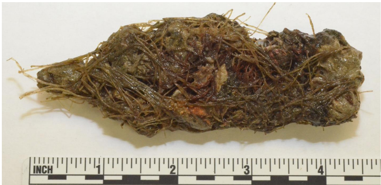
(b) Duplex 2205 Stainless Steel Coupon 8, Back Side
