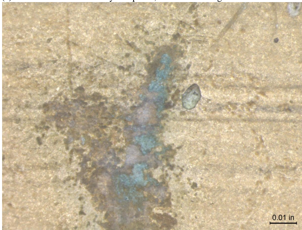
(b) Z-Alloy Coupon 1, Before Cleaning 50X
