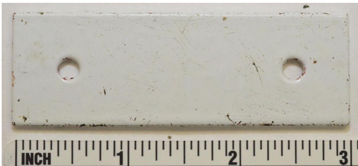
(b) Coated Duplex 2205 Stainless Steel Coupon 3, Back Side
