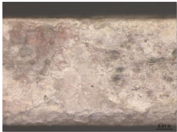
Photo 3-18. CDA 715 screen 2 at 50X magnification after cleaning.
