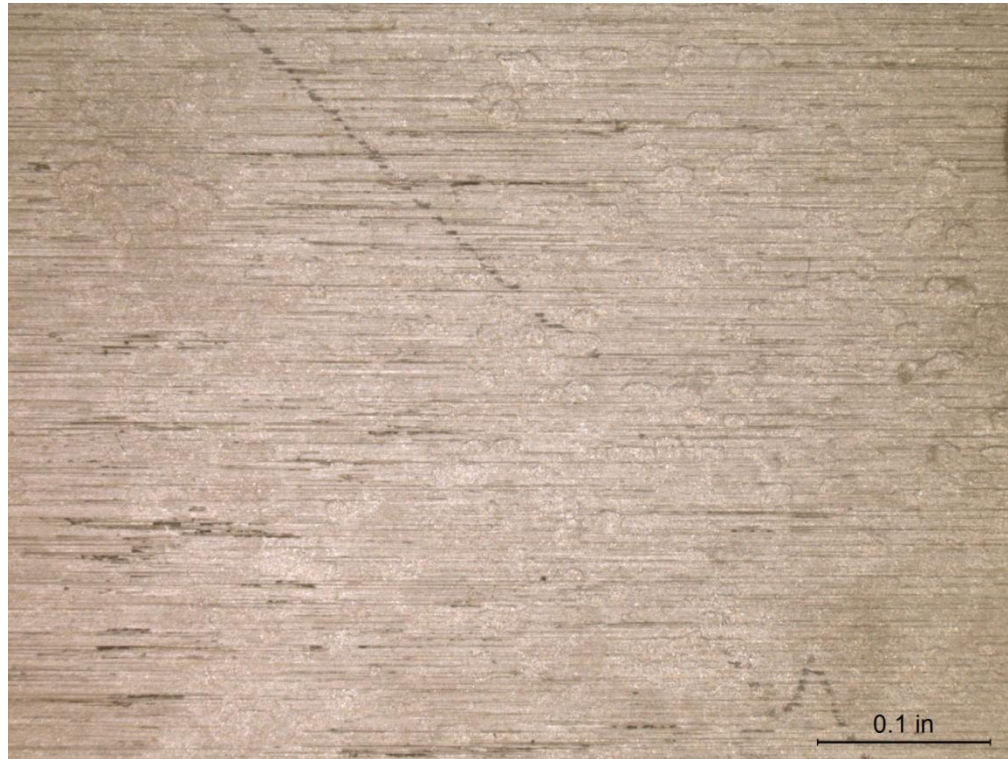
(a) CDA 706 Coupon 3, After Cleaning 10X
