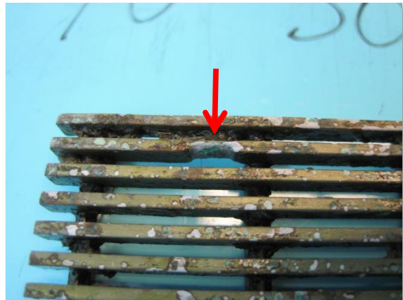
Photo 3-4. Coating damage to 2205 Duplex Stainless Steel wedge wire sample.
