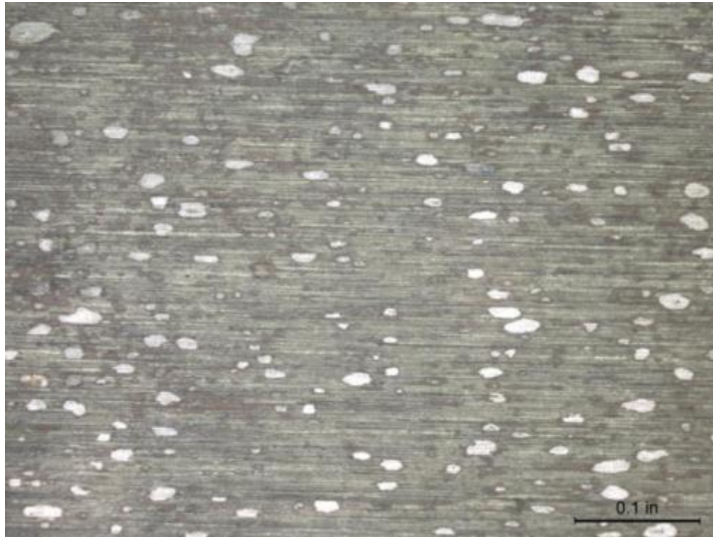
(a) CDA 715 Coupon 1, Before Cleaning 10X
