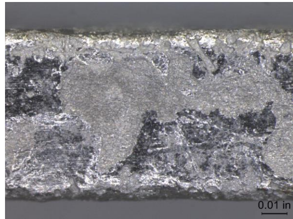
Photo 3-16. Detail view (50x) of 70-30 Cu-Ni wire screen, after cleaning.
