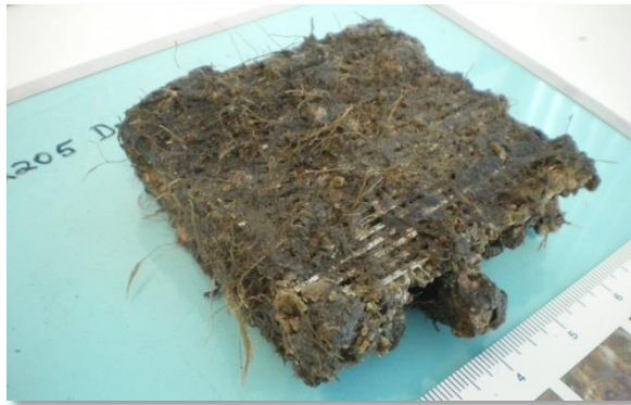
Photo 3-3. Marine life attached to uncoated 2205 Duplex stainless steel wedge wire screen.
