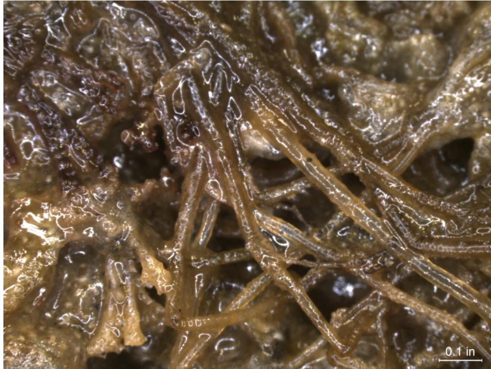
(a) Duplex 2205 Stainless Steel Coupon 8, Before Cleaning 10X
