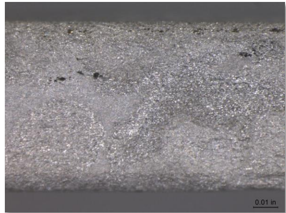
Photo 3-22. CDA 715 Screen at 50X magnification after cleaning.
