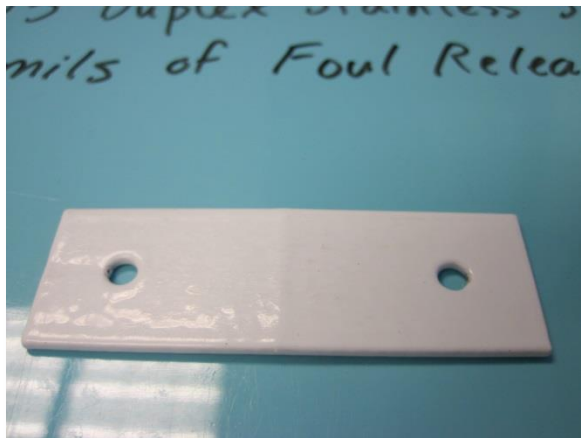
Photo 2-15. Coated 2205 Duplex stainless Steel 1-inch by 3-inch coupon with a weld.
