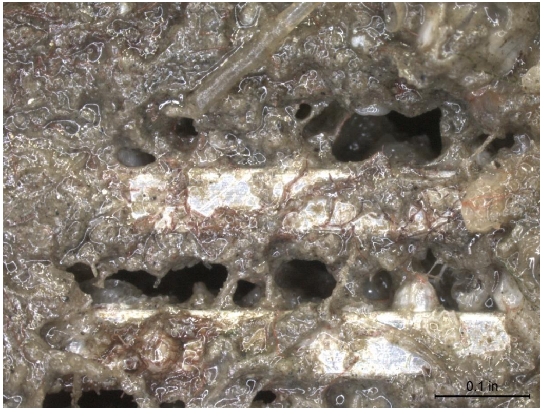
(a) Duplex 2205 Stainless Steel Screen 1, Before Cleaning 10X
