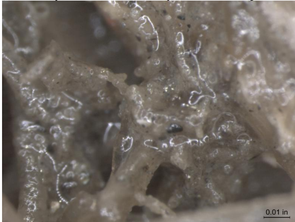
(b) Duplex 2205 Stainless Steel Coupon 7, Before Cleaning 50X
