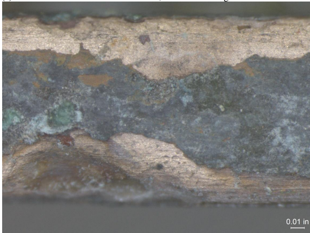
(b) CDA 706 Screen 3, Before Cleaning 50X
