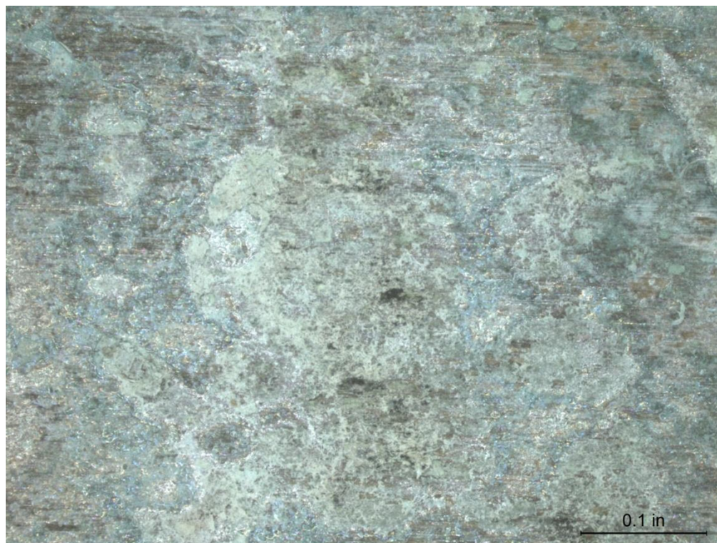
(a) CDA 715 Coupon 4, Before Cleaning 10X
