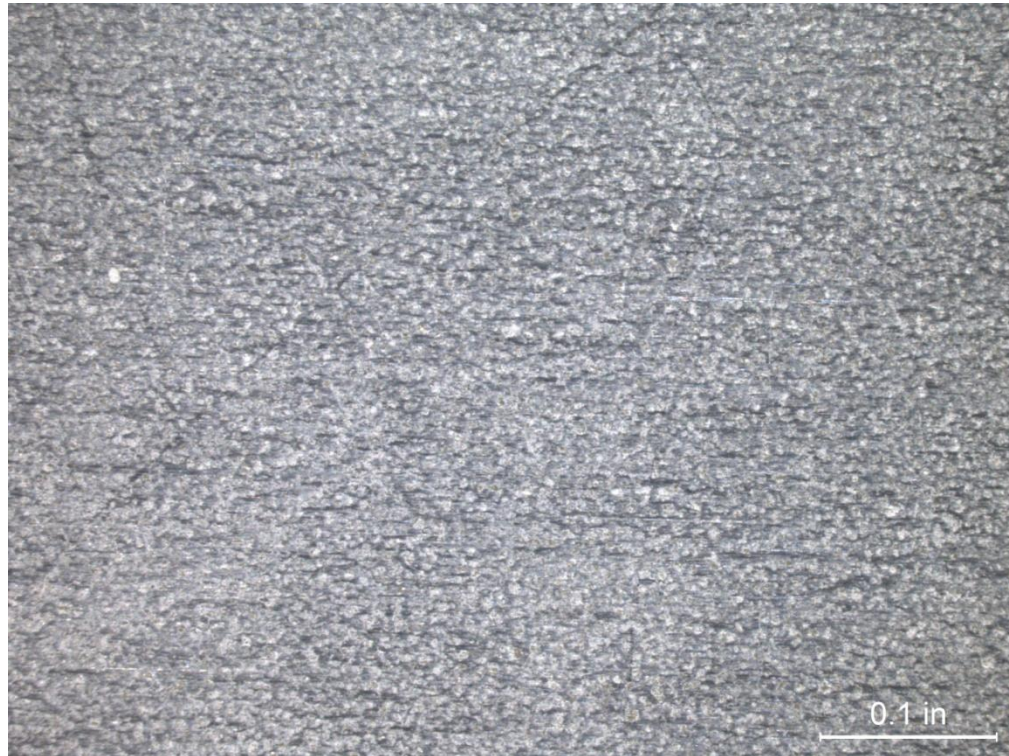
(a) Duplex 2205 Stainless Steel Baseline Plate 10X
