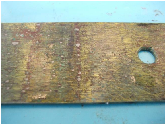
Photo 3-3. Minor damage to coating on edge of 2205 Duplex stainless steel coupon.
