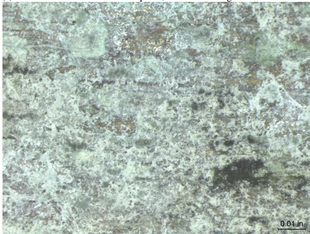
(b) CDA 715 Coupon 4, Before Cleaning 50X
