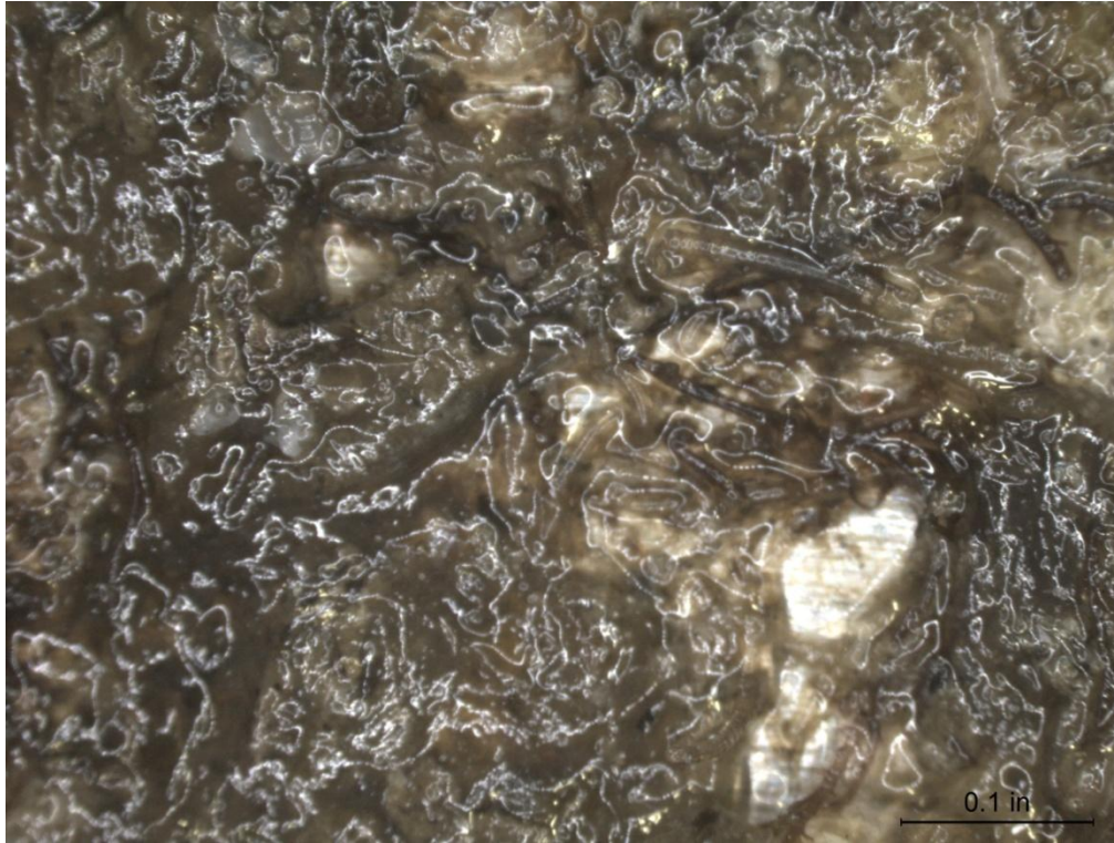
(a) Duplex 2205 Stainless Steel Coupon 9, Before Cleaning 10X
