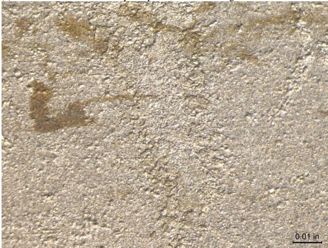
(b) Z-Alloy Coupon 1, After Cleaning 50X
