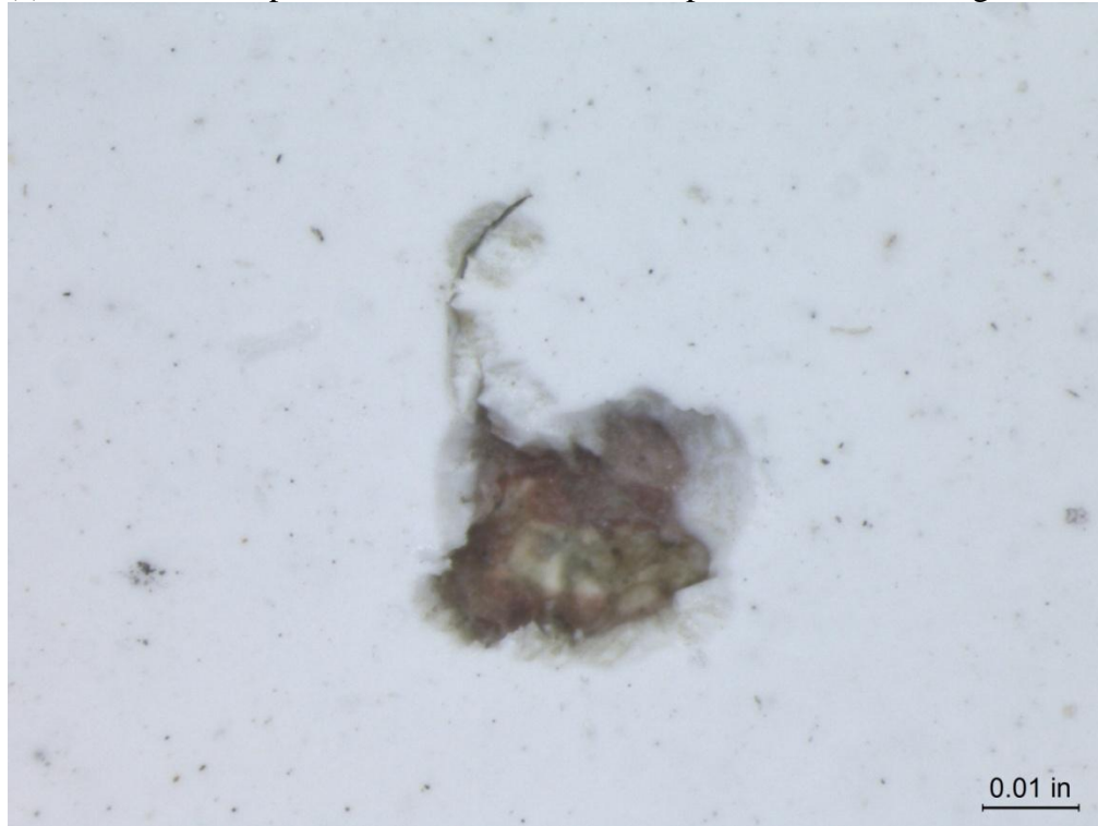
(b) Coated Duplex 2205 Stainless Steel Coupon 3, After Cleaning 50X
