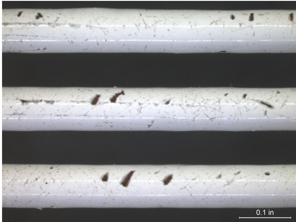
(a) Coated Duplex 2205 Stainless Steel Screen 4, After Cleaning 10X
