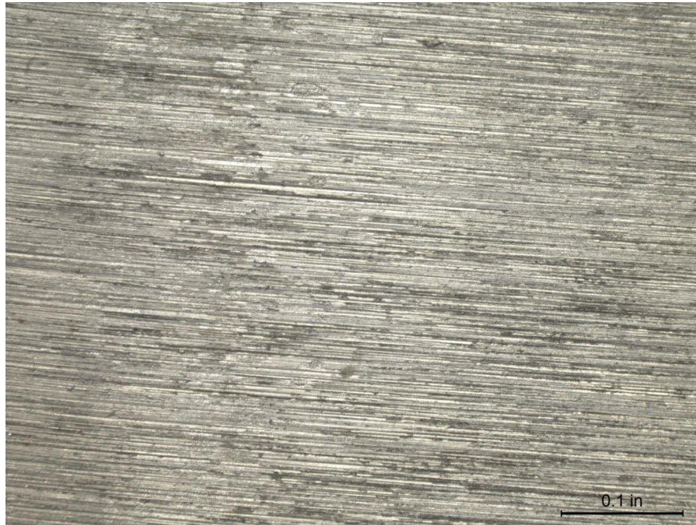
(a) CDA 715 Coupon 1, After Cleaning 10X
