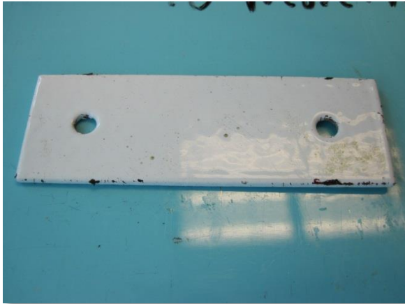
Photo 3-3. Minor damage to coating on edge of 2205 Duplex stainless steel coupon.
