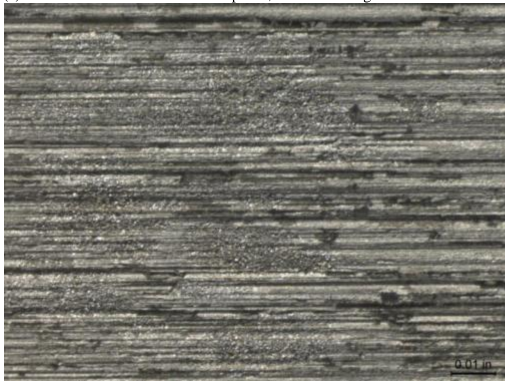
(b) CDA 715 Coupon 1, After Cleaning 50X
