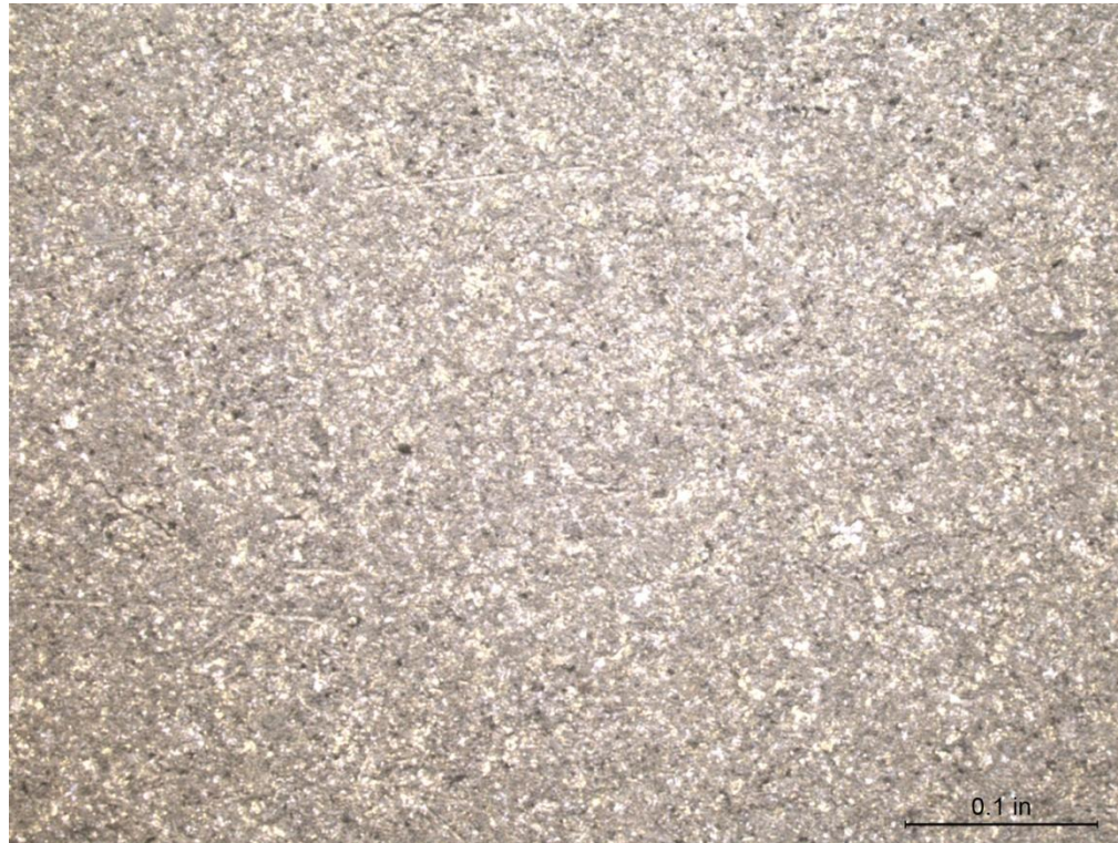
(a) Z-Alloy Plate, After Cleaning 10X
