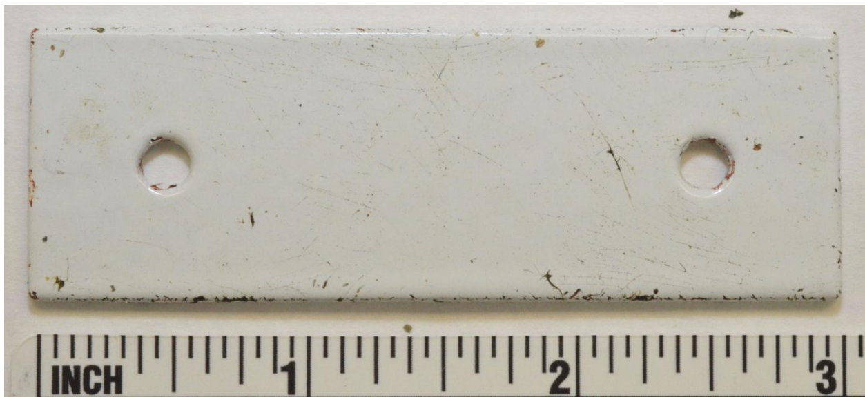
(b) Coated Duplex 2205 Stainless Steel Coupon 3, Back Side
