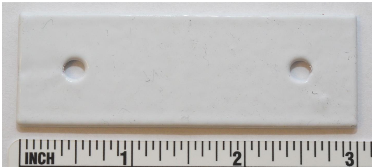
(b) Coated Duplex 2205 Stainless Steel Baseline Coupon, Back Side
