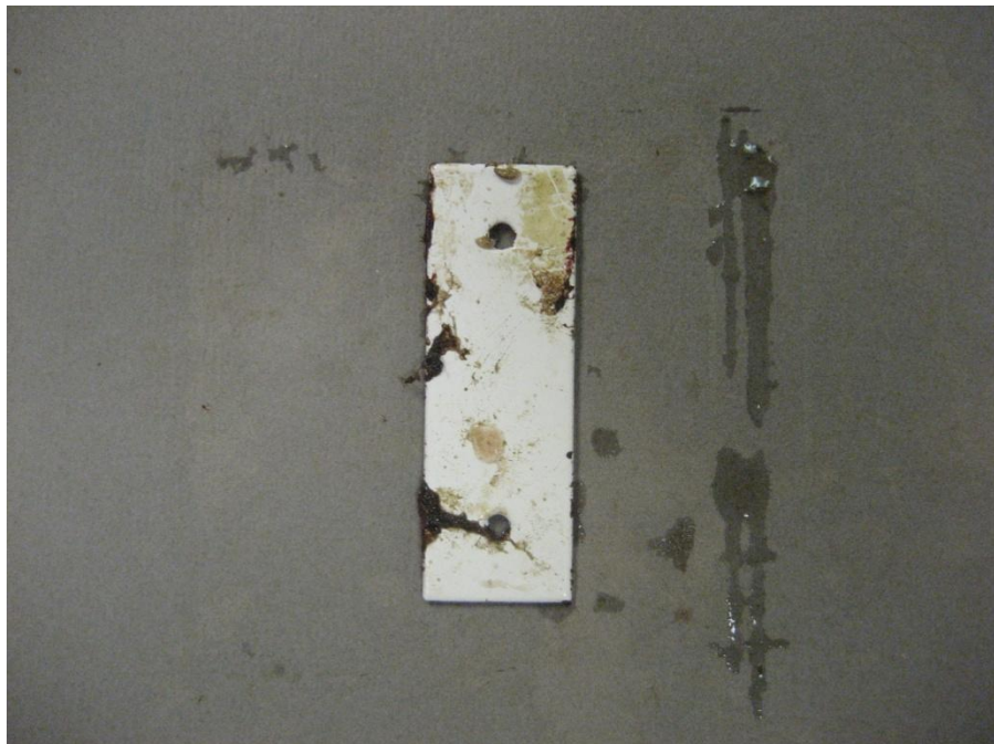
Figure 6. 2205 stainless steel coupon with foul release coating, photographed 04/22/15.
