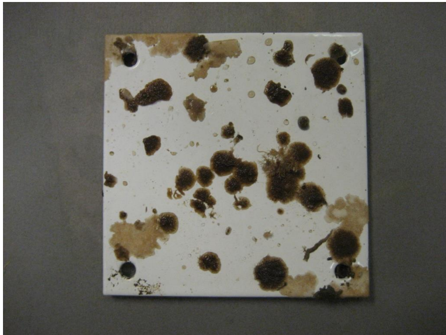
Figure 20. 2205 stainless steel test plate with foul release coating (Test Plate 5), photographed 06/18/15 prior to biofouling inspection.
