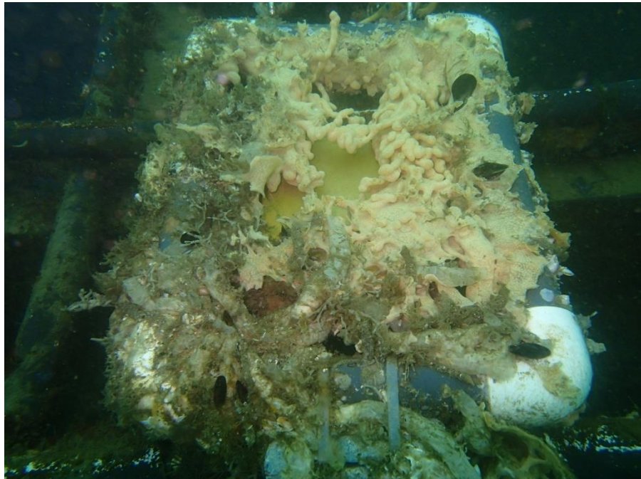
Figure 15. Z-alloy test plate and PVC frame (Test Plate 3), photographed 06/16/15 in situ after removal of its Vexar mesh bag.
