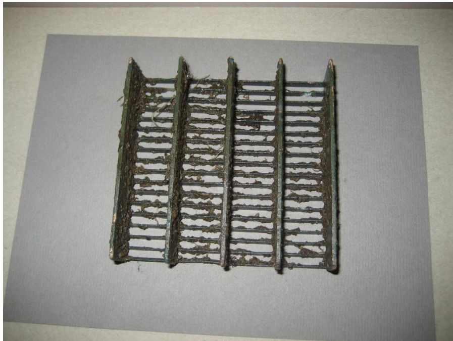
Figure 1. 90/10 Cu/Ni (CDA706) Wedgewire sample, photographed 04/22/15.
