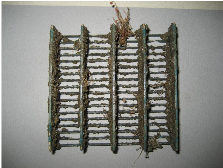
Figure 1. 90/10 Cu/Ni (CDA706) Wedgewire sample, photographed 06/17/15.
