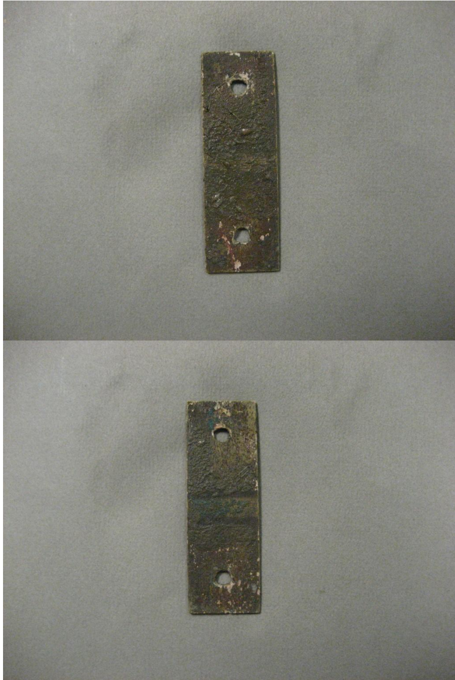
Figure 2. 90/10 Cu/Ni (CDA706) coupon, photographed 12/30/14.
