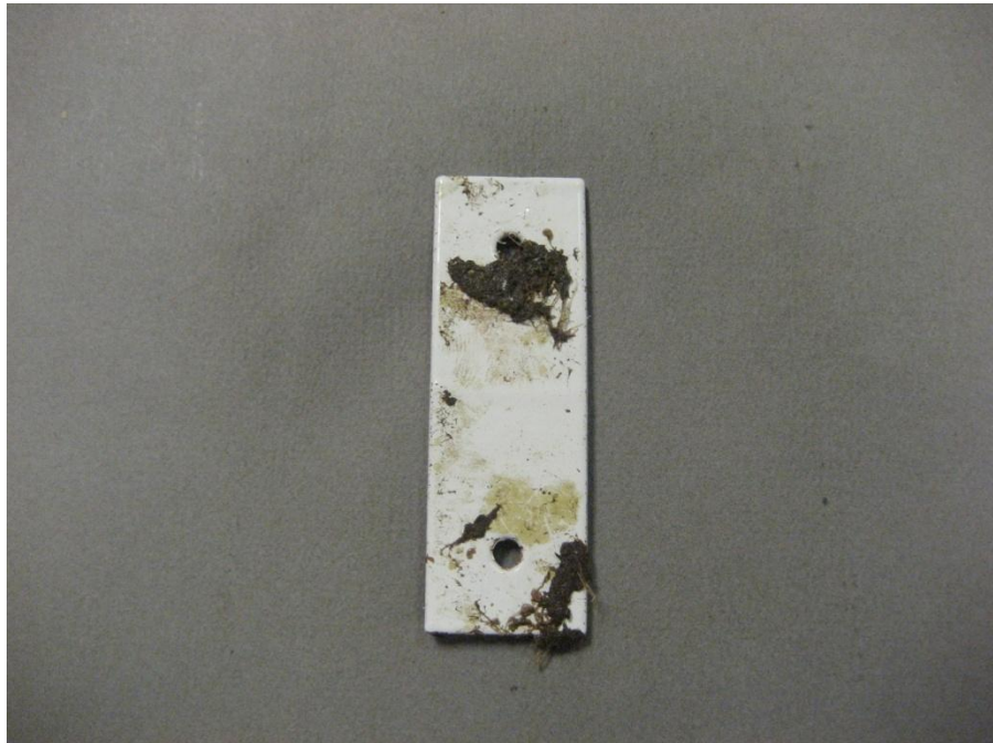
Figure 6. 2205 stainless steel coupon with foul release coating, photographed 12/30/14.
