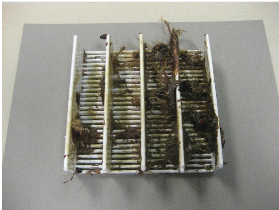
Figure 5. 2205 stainless steel Wedgewire sample with foul release coating, photographed 04/22/15.
