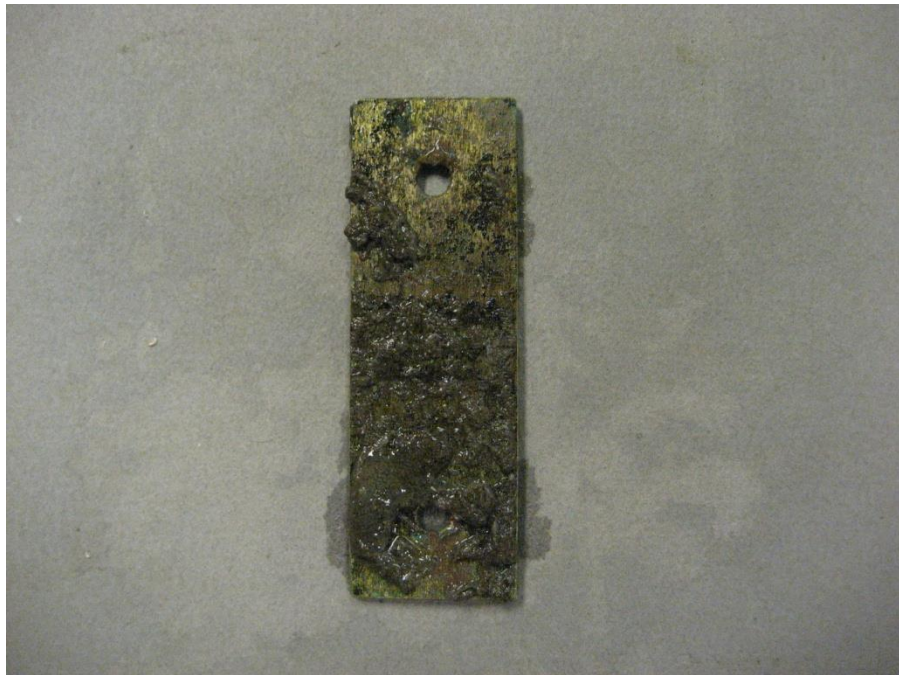
Figure 10. 70/30 Cu/Ni (CDA715) coupon, photographed 06/17/15.
