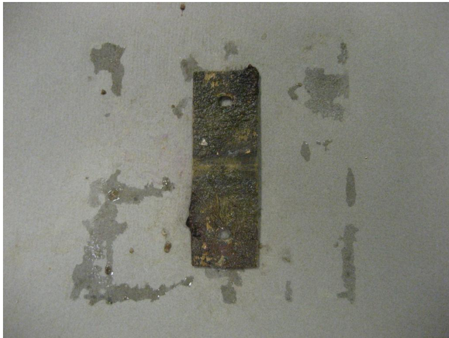
Figure 2. 90/10 Cu/Ni (CDA706) coupon, photographed 04/22/15.
