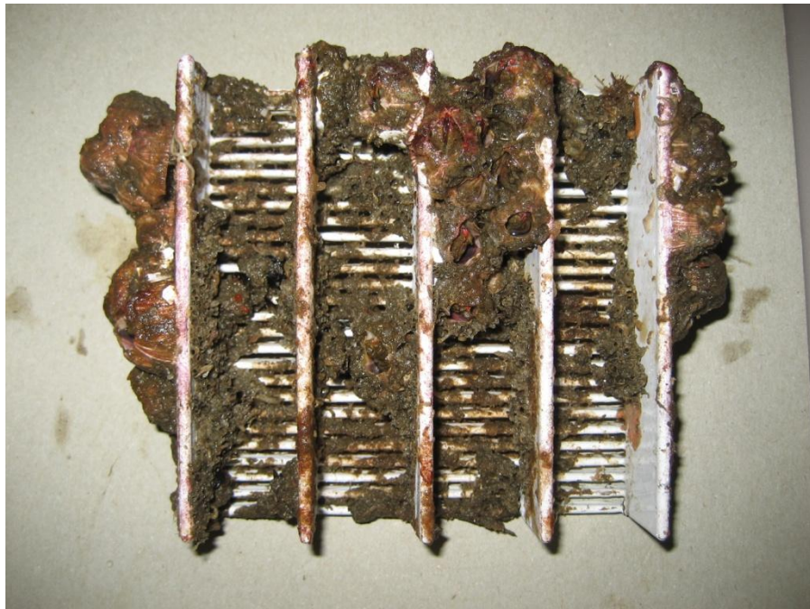
Figure 2. 2205 stainless steel wedgewire sample with foul release coating, photographed 05/24/17.
