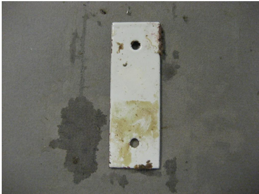
Figure 6. 2205 stainless steel coupon with foul release coating, photographed 06/17/15.
