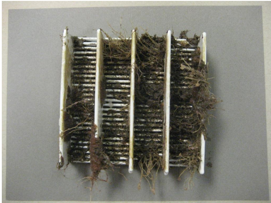
Figure 5. 2205 stainless steel Wedgewire sample with foul release coating, photographed 12/30/14.
