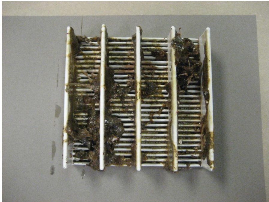
Figure 5. 2205 stainless steel Wedgewire sample with foul release coating, photographed 06/17/15.
