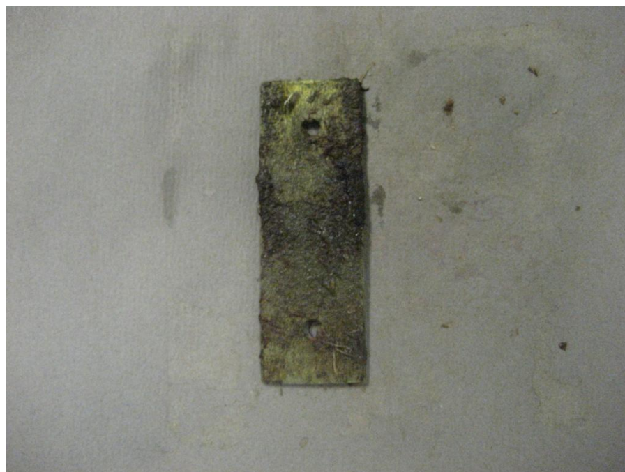
Figure 10. 70/30 Cu/Ni (CDA715) coupon, photographed 04/22/15.
