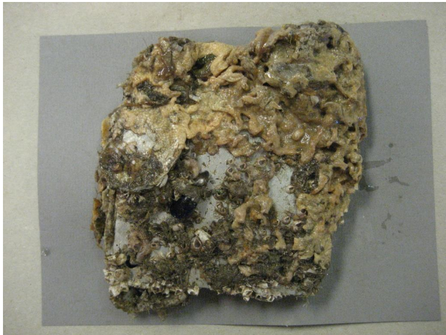
Figure 18. 2205 stainless steel test plate (Test Plate 4), photographed 06/18/15 prior to biofouling inspection.
