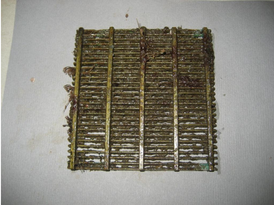
Figure 9. 70/30 Cu/Ni (CDA715) Wedgewire sample, photographed 04/22/15.
