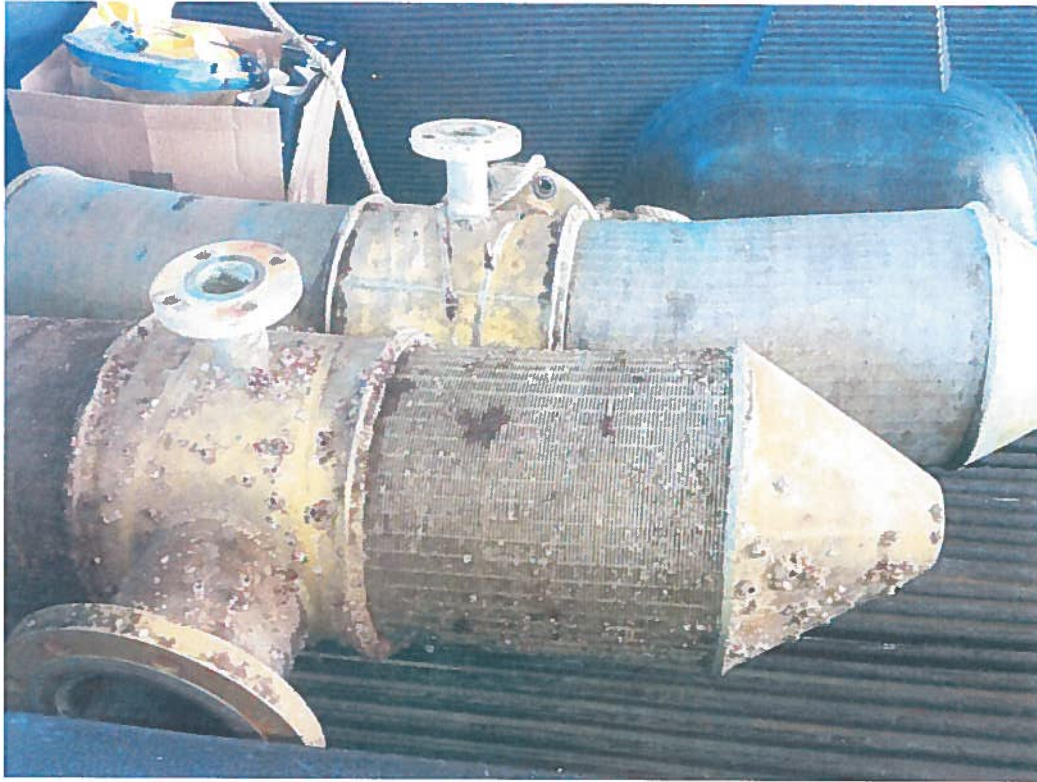
Figure 1. Wedge wire screens. Photo courtesy of Tetra Tech.
