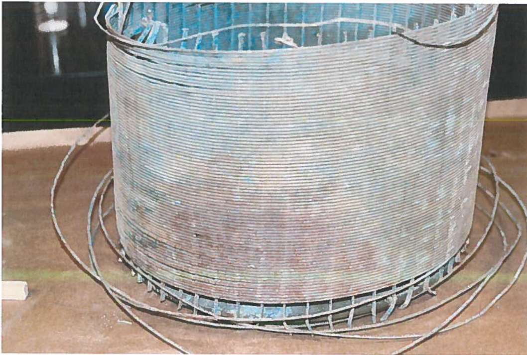
Figure 2. Wedge wire screen examined by Corrpro.
